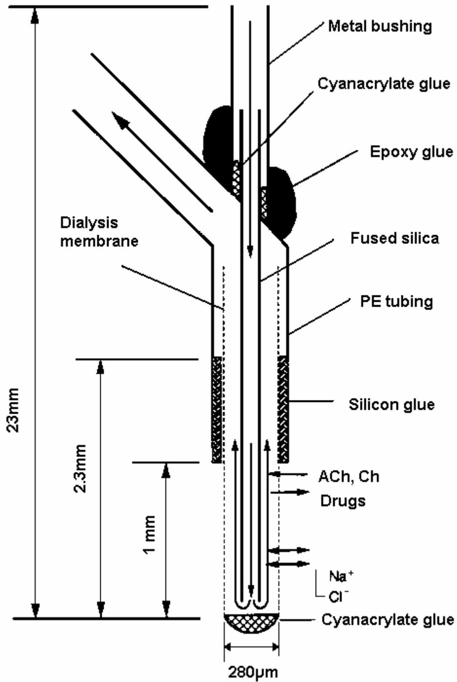
Figure 3.2: Schematic representation of a microdialysis probe (not to scale).
