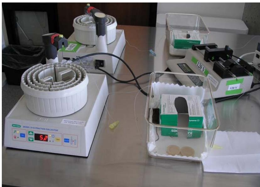
Figure 3.4: Microdialysis setup. Perfusion fluid is pumped from a syringe (top right) through PE tubing to the probe implanted in the mouse hippocampus (center). Outflow is transferred by another piece of PE tubing to the fraction collector (left). Up to four mice in parallel underwent perfusion (background).
