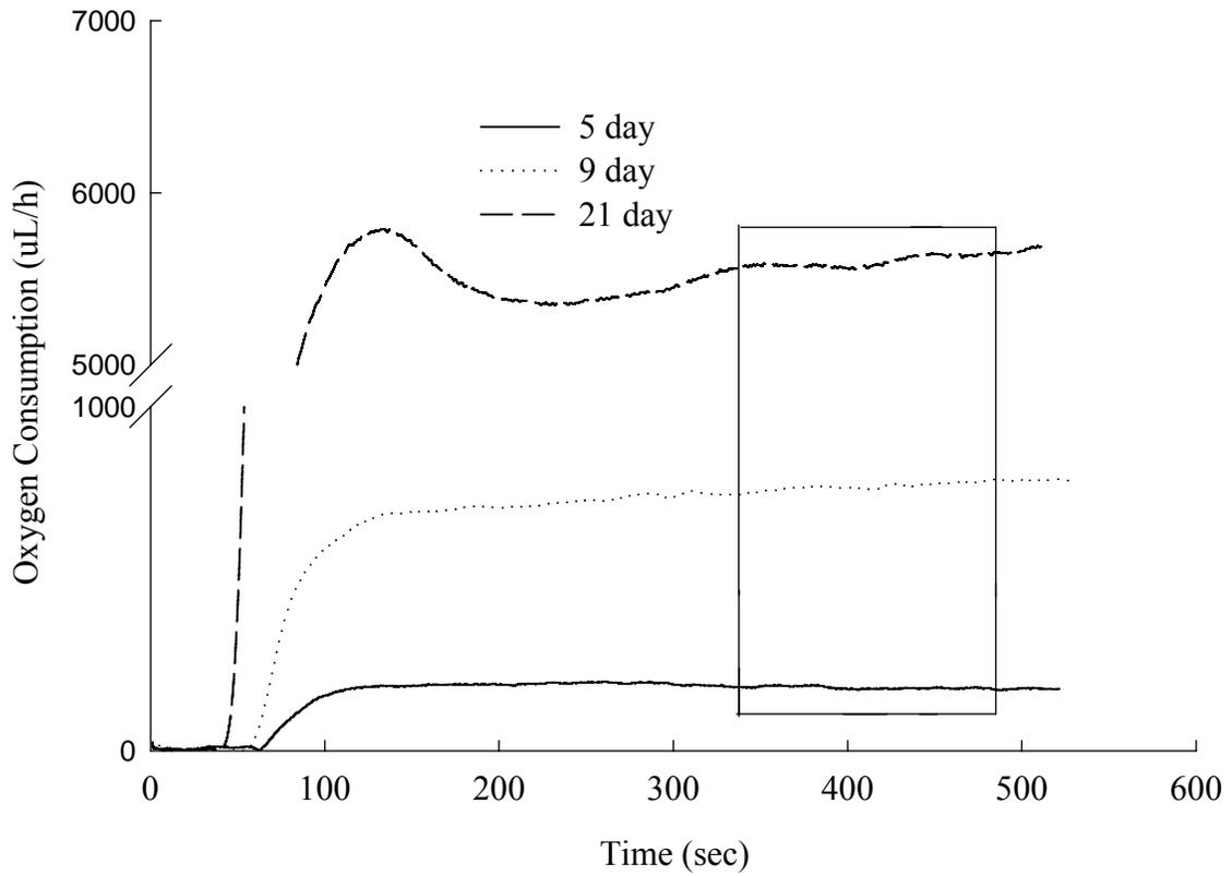
Figure 3.1. Representative graphs of oxygen consumption rates ( $\mu\text{L/hr}$ ) by 5, 9, and 21 days old northern bobwhite quail eggs. The box represents a data collecting window of 120 s after achieving a plateau.
