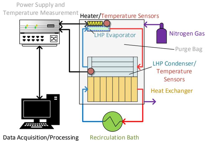
**Figure 7. Step 1 testbed configuration.**
