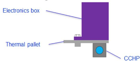
**Figure 3. Cross section of thermal pallet showing representative configuration.**
