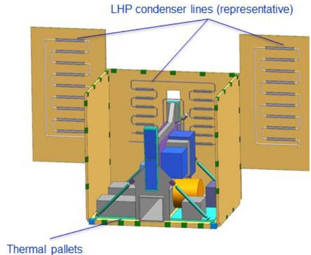
**Figure 2. K-PLM layout with representative thermal hardware configuration.**
