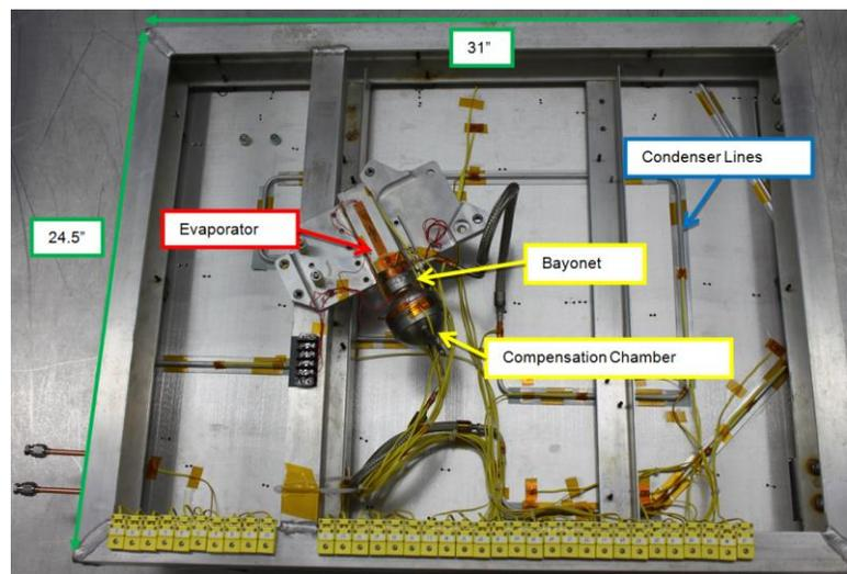
**Figure 6. TES LHP Engineering Model modified for SWOT LHP Step 1 testbed.**
