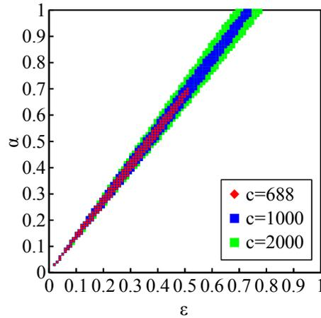
**Figure 2. Combinations of solar absorptivity and infrared emissivity on outside surface of micro satellite that keep temperature of micro satellite within allowable temperature range under worst cold case and worst hot case. Solar absorptivity and infrared emissivity are calculated at the intervals of 0.01.**
