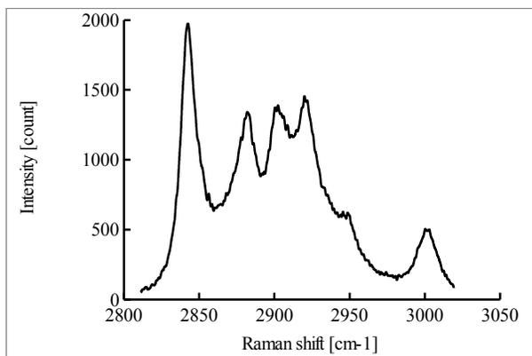
**Figure 7. Raman shift of CH<sub>2</sub> band of trans-1,4-polybutadien in Figs.4-6.**
