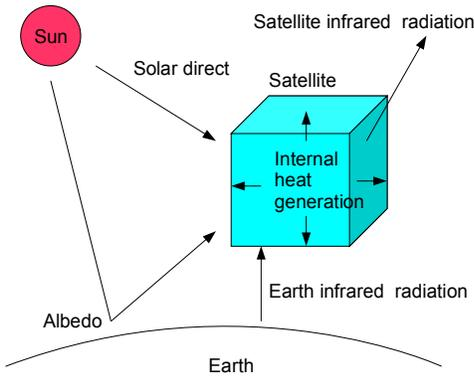
**Figure 1. Schematic of heat input to satellite and heat output from satellite.**
