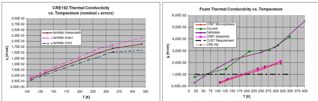
Figure 3 . Thermal Performances of ETI (CRE 192 and comparison with current foams)
