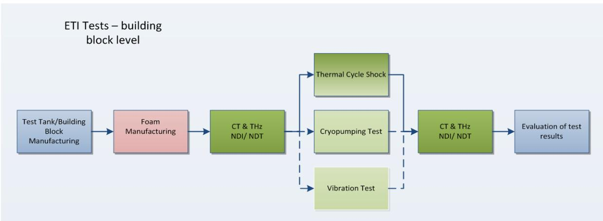
Figure 6. Flow plans for Cat . 5. and 6. Tests shown as example for IWTI for breadboard samples, for ETI on building block level
