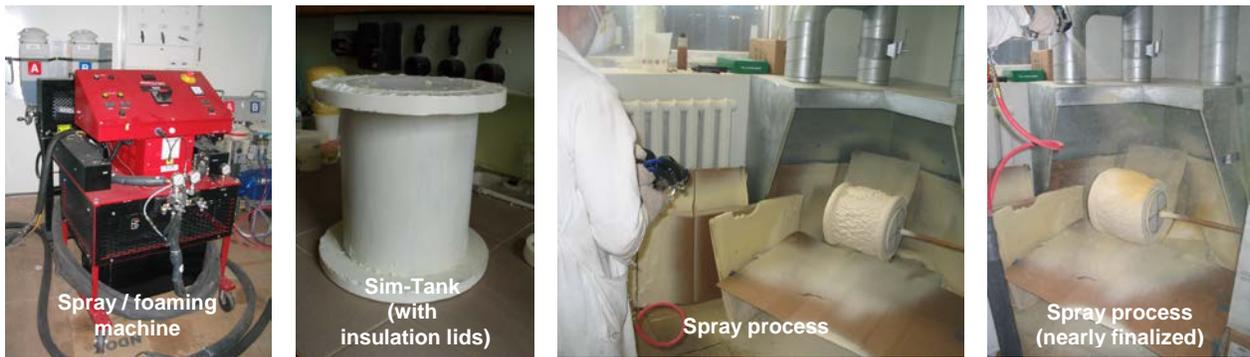
**Figure 4 . Foam spray-on process (illustrated here for a small simulation tank)**
