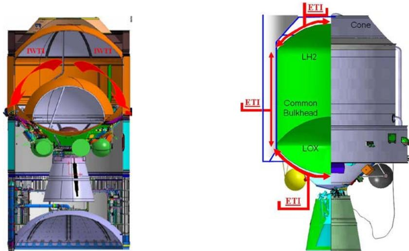
Figure 1 . Locations of IWTI & ETI Insulation on current LH2 & LOX Tank Configurations for Upper Stage
