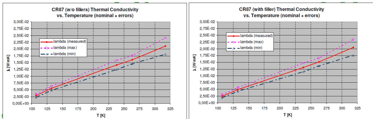
**Figure 2 . Thermal Performances of IWTI (bare and with microsphere filler)**
