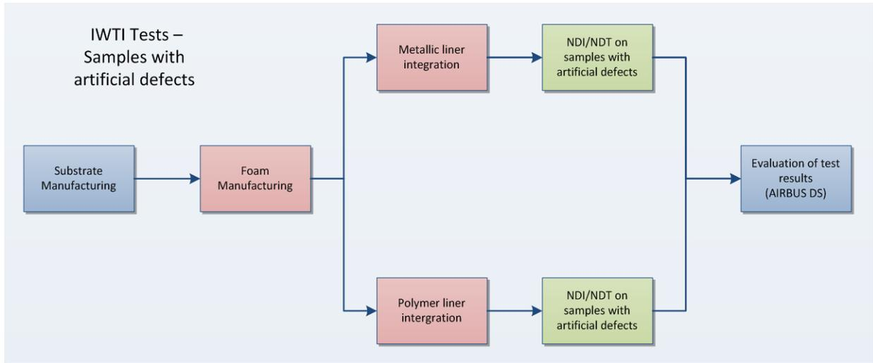
**Figure 8. Flow plan for NDI Specimens with artificial Defects**
