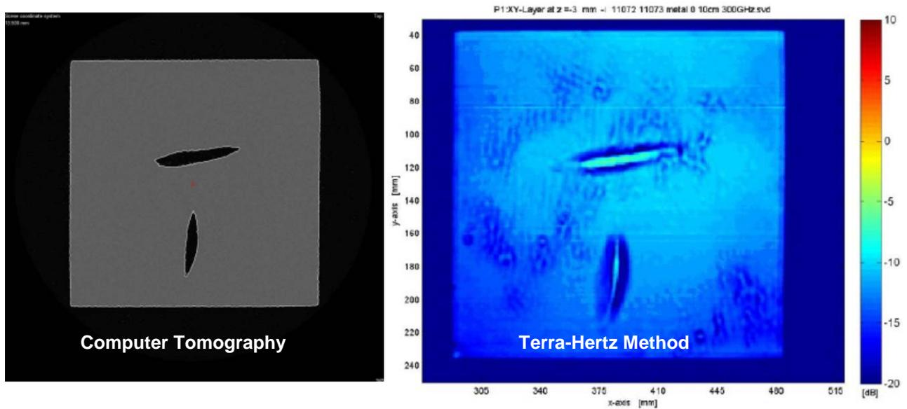
**Figure 9. Typical NDI Results for lab (CT) and field (Terra-Hz) scale methods (type of defect: voids)**
