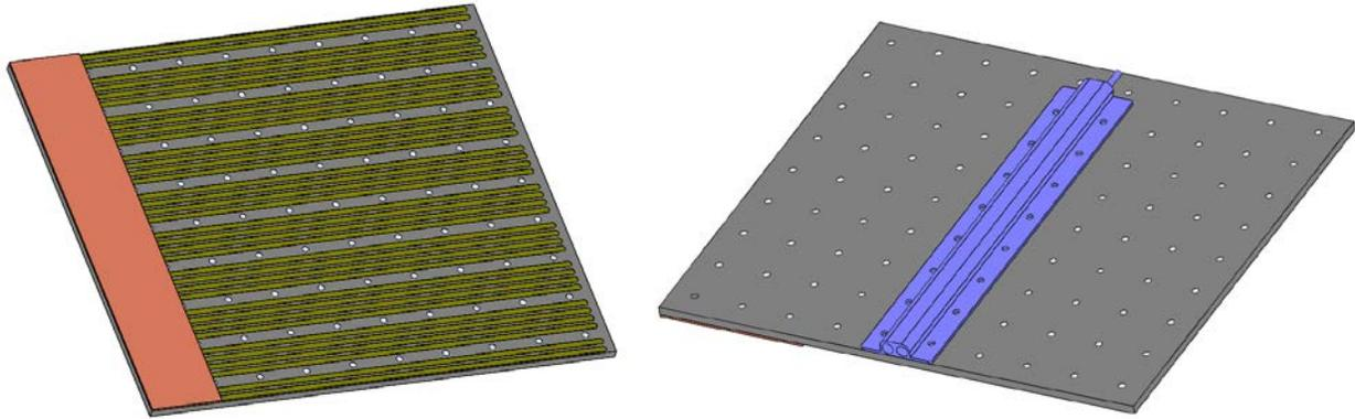
**Figure 13.** With the CCHP evaporator located in the center of the plate. 175 W (0.51 W/cm<sup>2</sup>) was applied over a 7.6 x 35.7 cm (3 x 18 in.) strip at the edge of the plates.
