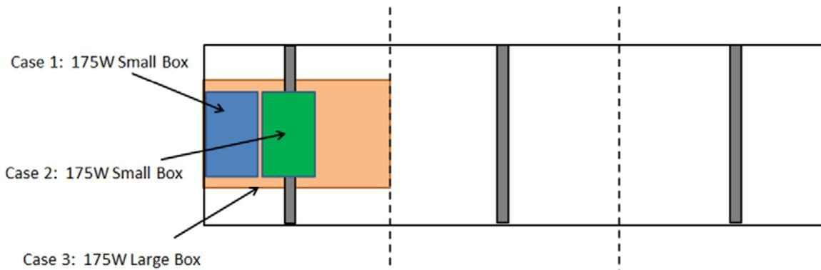
Figure 6: Heat load conditions used in thermal analysis
