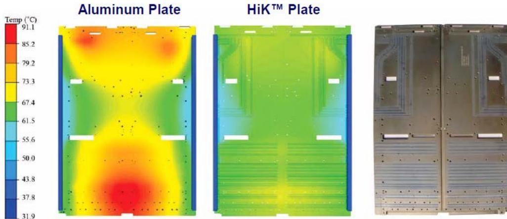
**Figure 3.** In one example, HiK™ plates showed an experimental reduction of  $22^{\circ}\text{C}$  in peak temperature compared to a baseline aluminum plate. (a) Aluminum plate thermal analysis. (b) HiK™ plate thermal analysis. (c) HiK™ plate. Note that the heat pipes are tailored based on the electronics locations to give the maximum effective thermal conductivity.
