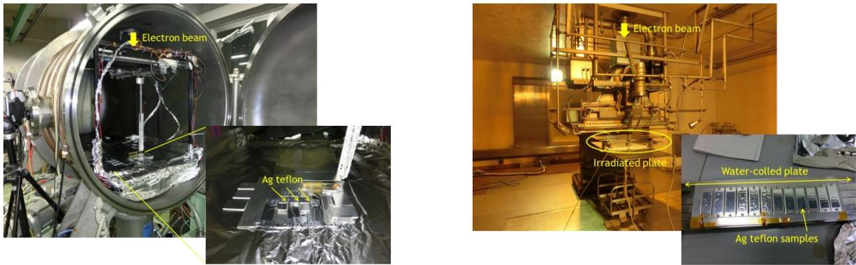
**Figure 4. Test setup for low-energy electrons (left) and high-energy electrons (right)**
