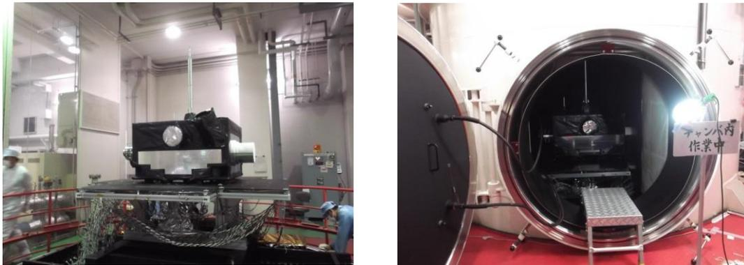
Figure 7. Thermal balance test configuration
