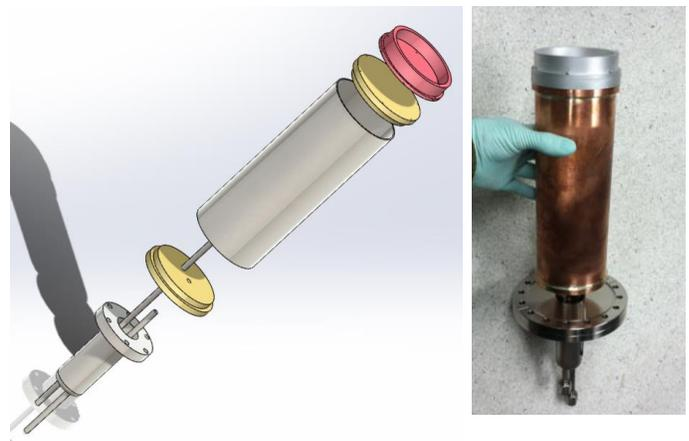
**Figure 7. Internal dewar: exploded view and photograph.**
