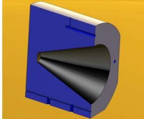
**Figure 14. Cross section of conical cavity.**
