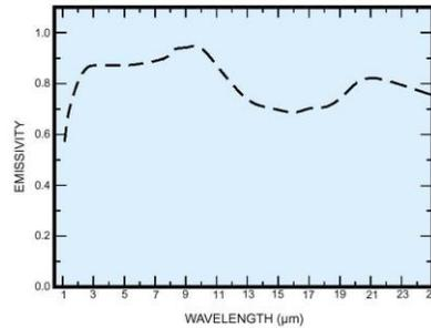
**Figure 19. compact IR emitter used for preliminary testing and spectral emissivity plot<sup>14</sup>.**
