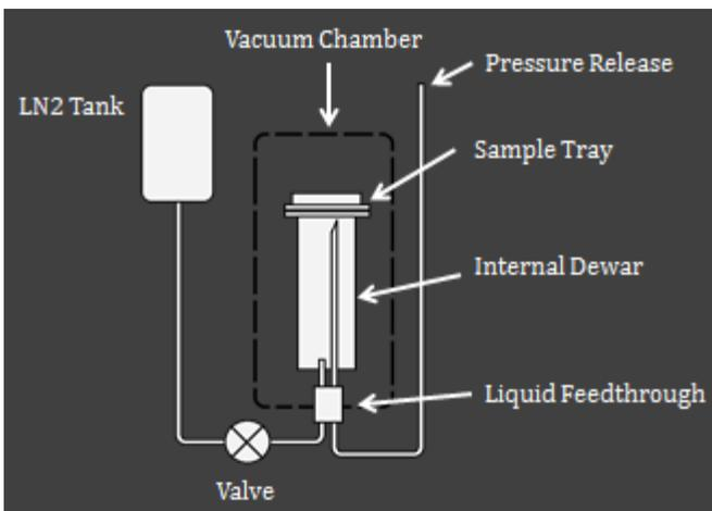
**Figure 6. Gravity feed.** This schematic shows the internal dewar setup.
