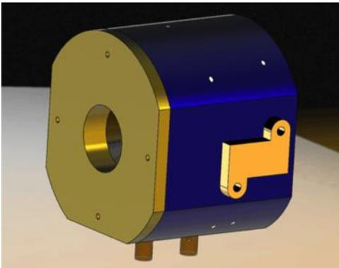
**Figure 15. Cavity component with aperture and resistor.**
