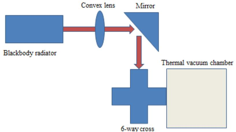
**Figure 17. Diagram of external testing setup.**
