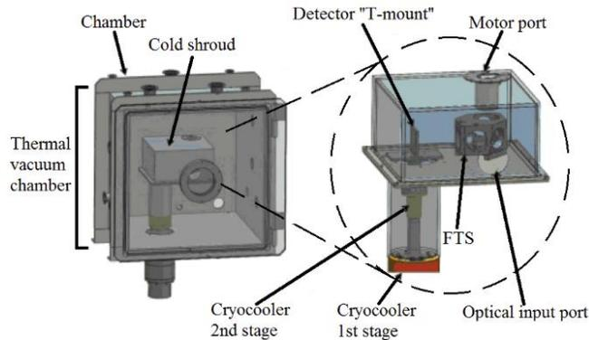
**Figure 3. Components of the vacuum chamber.**
