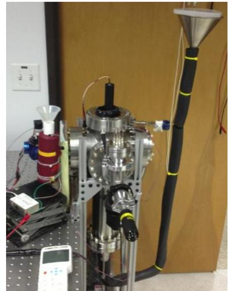
**Figure 18. Sample apparatus setup with benchtop version of CIRIS spectrometer.**
