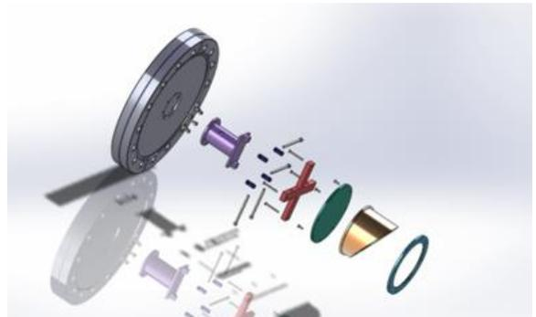
Figure 9. Exploded CAD view of the mirror assembly.
