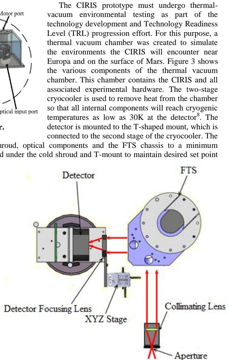
**Figure 4. Optical setup within the vacuum chamber.**
