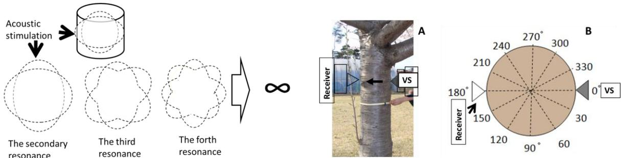
Fig. 3 The method of acoustic vibration analysis. The basic vibration track according to the theory in the case of the column shape object given an acoustic stimulation (Left side) and the method for the acoustic vibration analysis (A) and the position (B) in this study. An acoustic stimulation by vibration speaker (VS) is received by the receiver (Right side).
