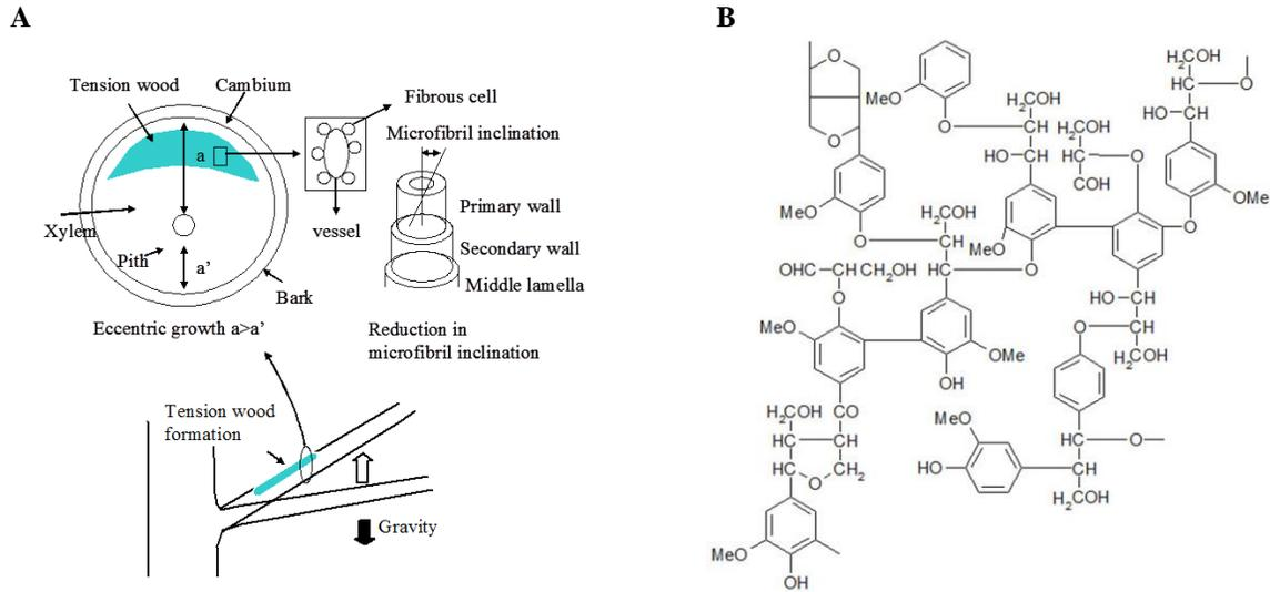
Fig. 2 Tension wood formation in angiosperm;A, and an example of the component of lignin;B.
