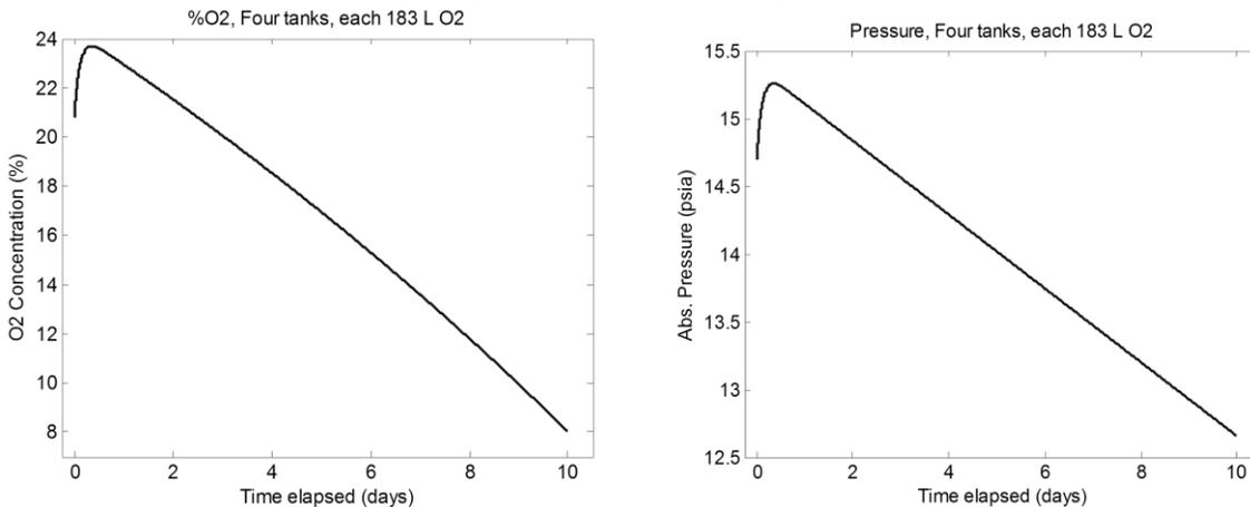
**Figure 5. Simulated O<sub>2</sub> concentration and absolute pressures as a result of a 183 L O<sub>2</sub> supply venting through 25-micron flow-restricting orifice into a sealed cabin with 4m<sup>3</sup> of free air volume.**
