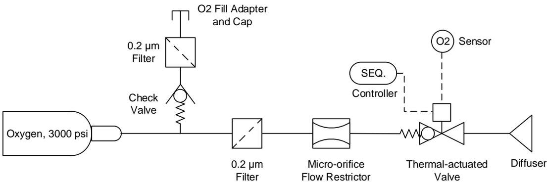
**Figure 3. AEM-E oxygen system design, with high-pressure flow restrictor, no pressure regulator, and custom-designed, thermally-actuated valve.**
