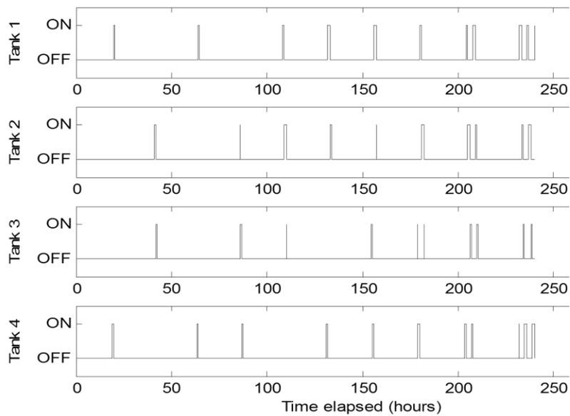
**Figure 13. Simulated valve actuation tests from predicted mission simulations.**
