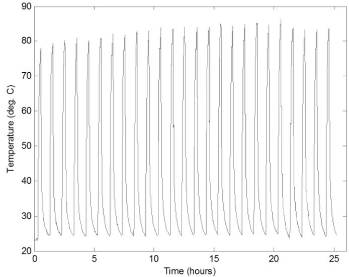
**Figure 12. Temperature history during valve actuations, with ambient air circulation.**
