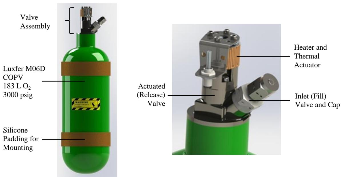
Figure 7. Cylinder assembly and valve assembly with major oxygen system components identified.
