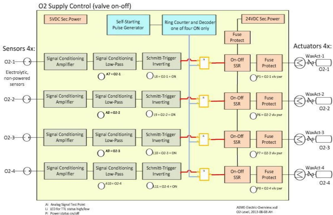
**Figure 8. Functional block diagram for the 4 independent oxygen release systems. Each of the 4 systems has its own dedicated partial pressure sensor, signal conditioning system, and associated valve control switch. A so-called digital ring counter ensures that only one of the 4 systems is enabled to release oxygen.**
