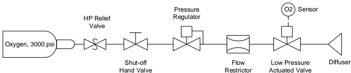
**Figure 1. Standard conventional approach to high-pressure oxygen delivery system design.**
