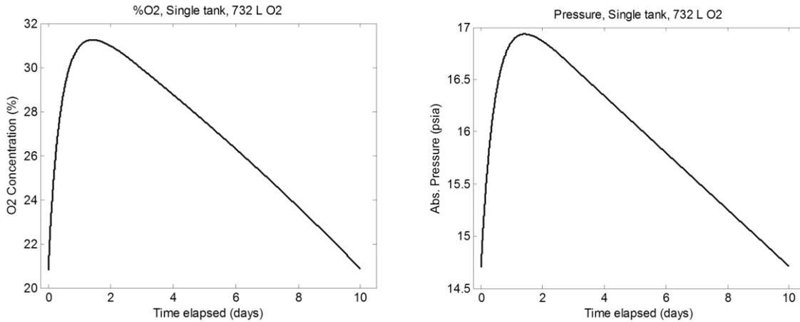
**Figure 4. Simulated O<sub>2</sub> concentration and absolute pressures as a result of the entire 732 L O<sub>2</sub> supply venting through a 25-micron flow-restricting orifice into a sealed cabin with 4m<sup>3</sup> of free air volume.**
