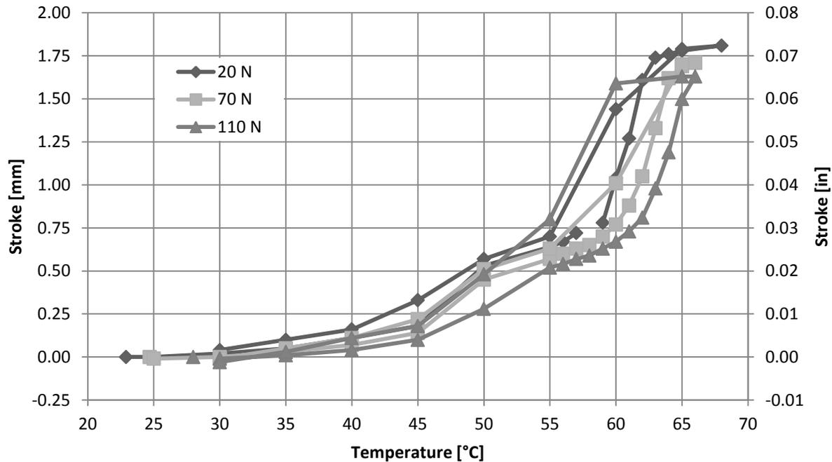
Figure 6. Experimental stroke distance measurements at various temperatures and preload forces.
