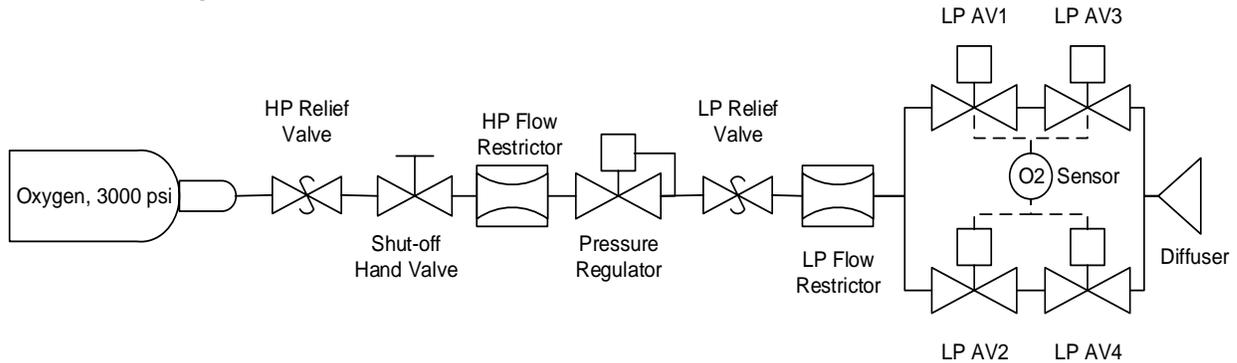
**Figure 2. Single fault-tolerant oxygen system design, with high-pressure flow restrictor.**
