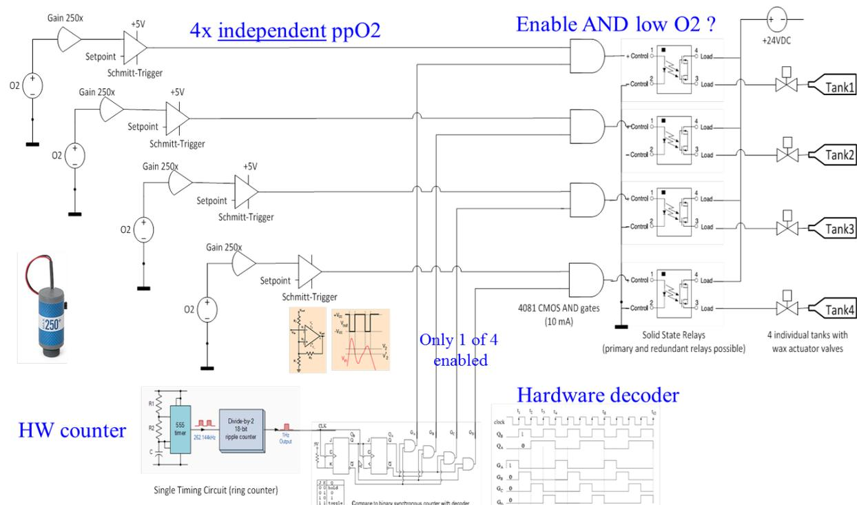
**Figure 9. The analog control system ensures that only one of the 4 valves can be enabled, and that only one system can release oxygen if it is enabled and senses low oxygen. The employed logic chips are very robust and no software or microprocessors are employed in this design. All setpoints are hard-wired.**
