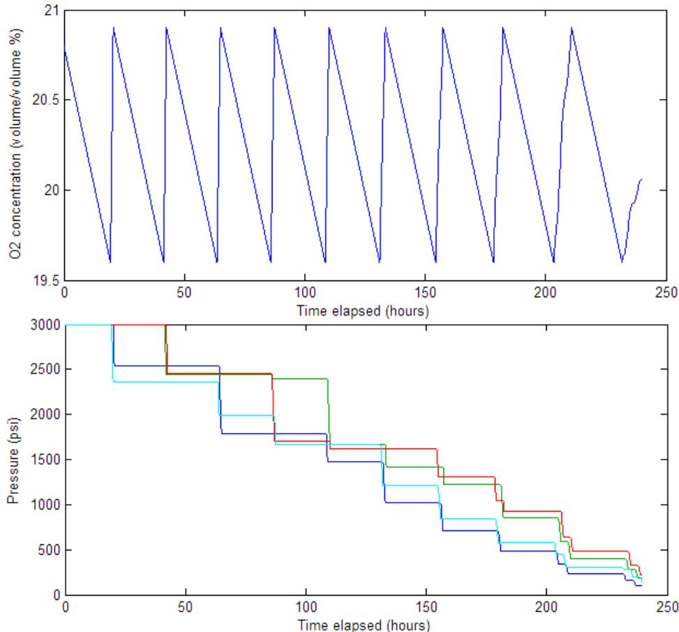
**Figure 14. Simulated environment and oxygen system performance over 10-day mission. O<sub>2</sub> concentration in the environment and pressure remaining in each of four cylinders are shown.**
