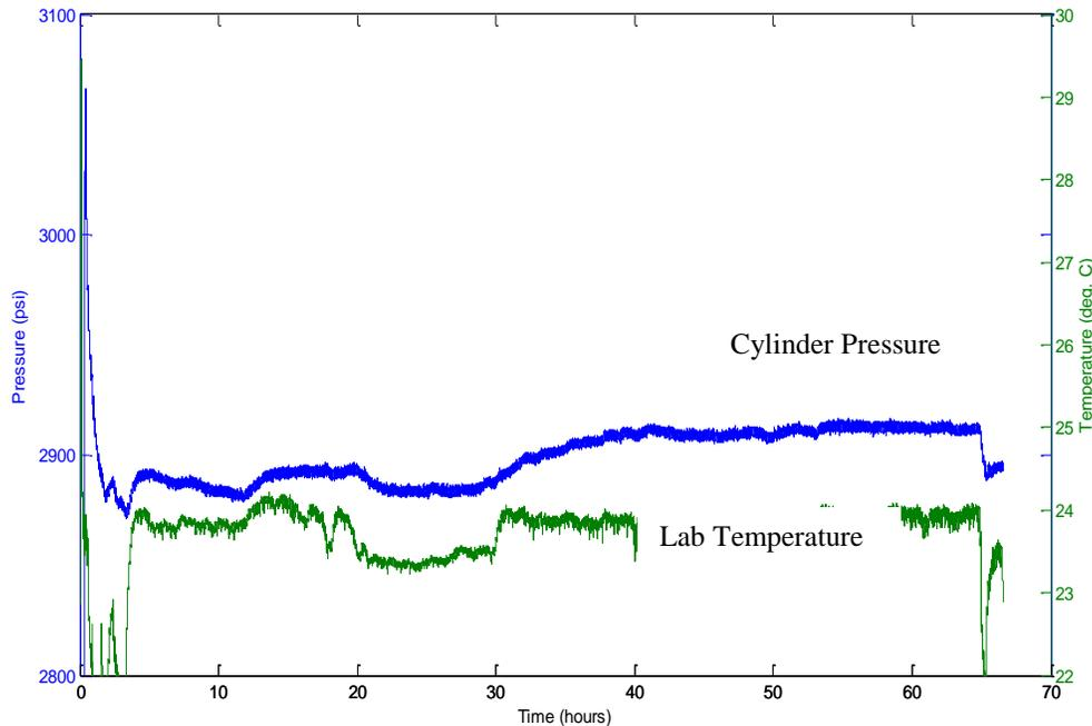
**Figure 10. Pressure history and leak rate determination over time from fill to end of test (68 hours).**
