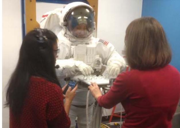
**Figure 9. Evaluating protocols for assessments of glove mobility. Test subject in pressurized suit performing “Pin” task.**
