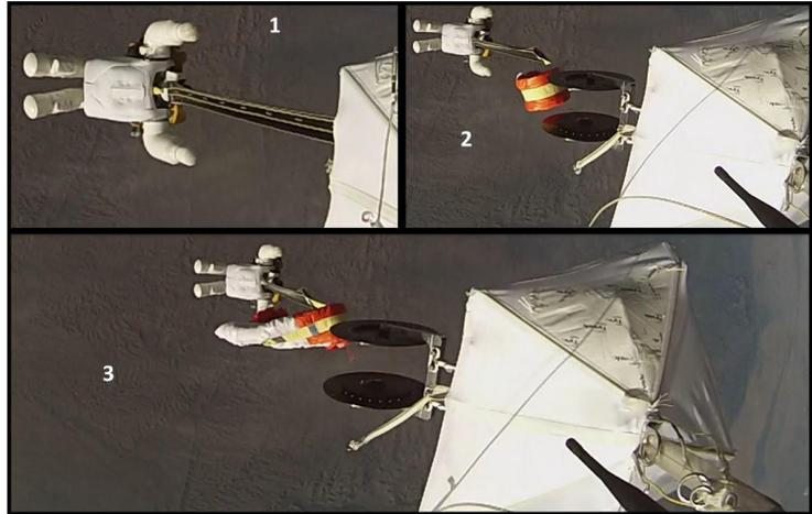
**Figure 2. SAEBER System:** *Deployed drogue pole does not tangle on rotating test article in free fall.*
