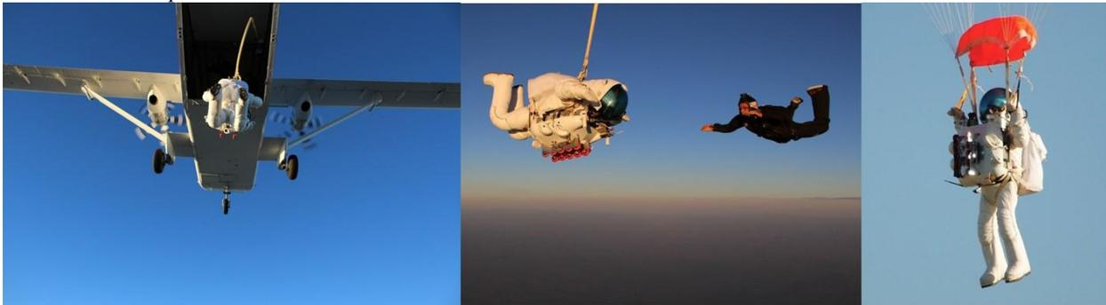
**Figure 11. Airplane Jump Tests:** *Left, Exiting the plane; Middle, Drogue descent; Right, Parafoil flight*
