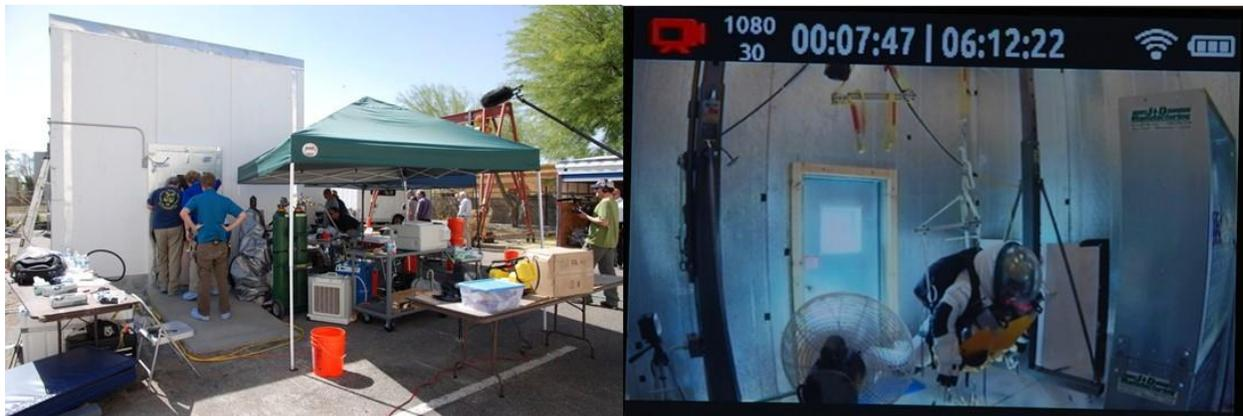
**Figure 9. Thermal – Cold Testing in the FRANKENFREEZER:** Left, testing underway under careful supervision of the team; Right: at 57°C (-70°F) a simulated altitude of 20 km (65,000 ft)
