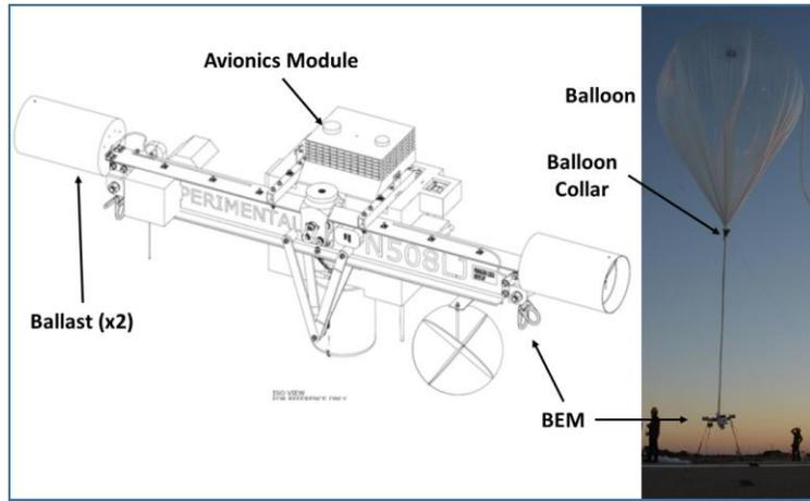
**Figure 3. Flight Vehicle: Balloon and Balloon Equipment Module (BEM)**
