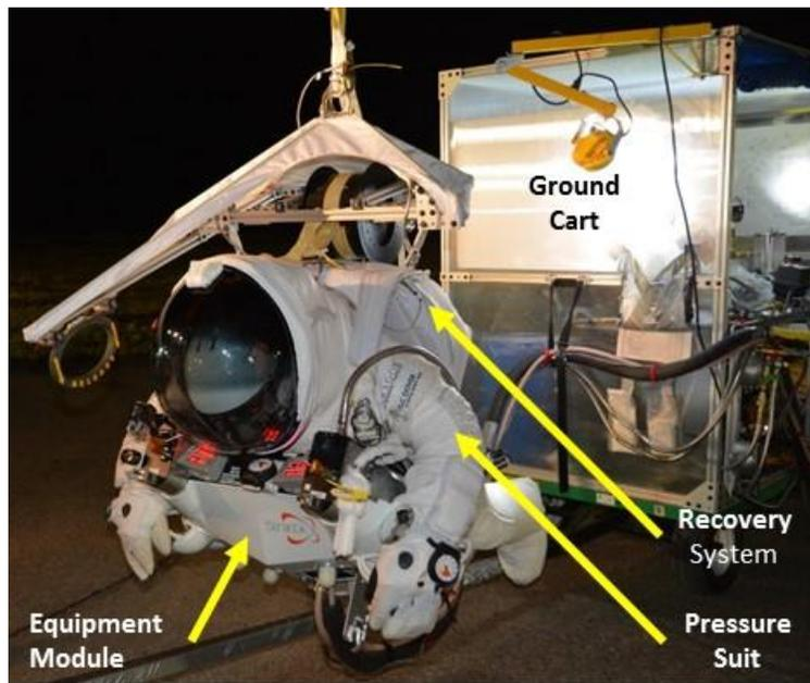
**Figure 1. Space Suit Assembly & Ground Cart.** During transport from the suit-donning facility to the launch site.
