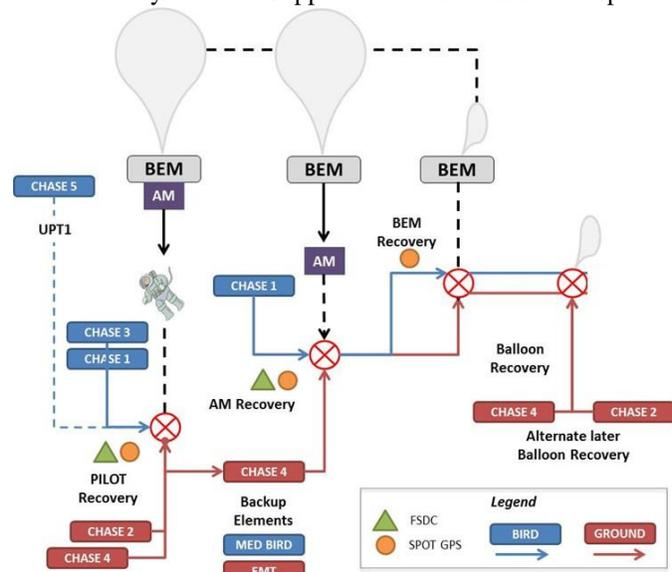
Figure 4. Chase ConOps Schematic
