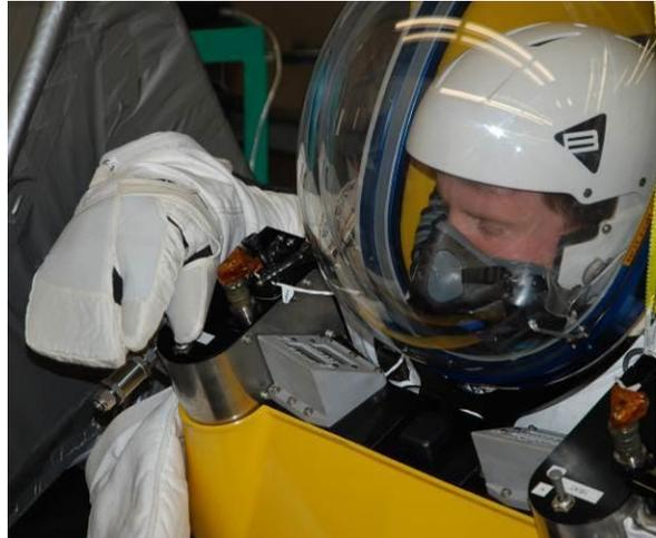
**Figure 7. Testing pilot access to the purge valve<sup>6</sup>.**
