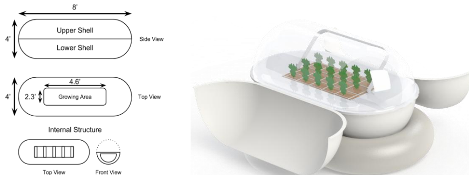
Figure 2. Structural ribs and shell (left) and CAD structural concept (right). The structural ribs are depicted in the lower ‘Top View’ drawing.
