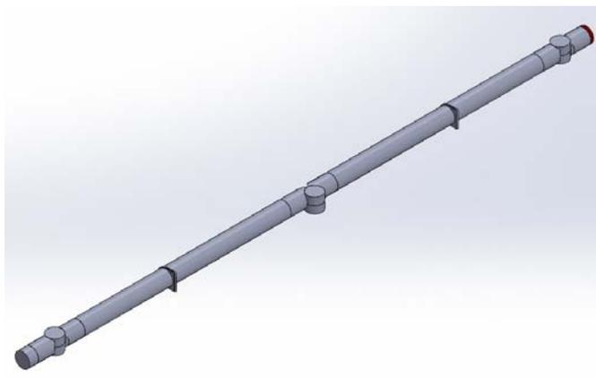
Figure 15. Folding 7DOF manipulator concept for SNC Dream Chaser (full extension)
