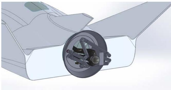
Figure 17. Dream Chaser contingency airlock egress with dual manipulators in launch configuration
