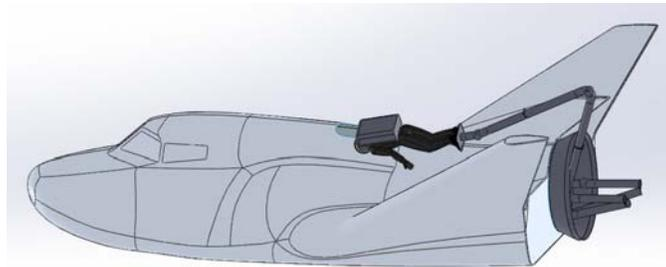
**Figure 19. Dream Chaser manipulator providing translation path for EVA egress from ground access hatch**
