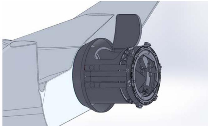
Figure 20. Rigid airlock with pre-mounted manipulators attached to aft bulkhead on LVIS structure
