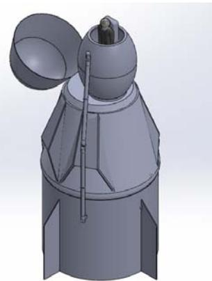
Figure 13. Inflatable airlock concept for SpaceX Dragon spacecraft
