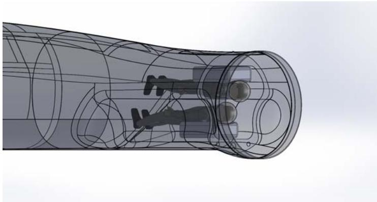
Figure 12. Concept for SNC Dreamchaser internal airlock configuration
