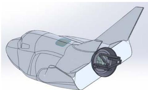
Figure 16. Dual manipulator launch stowage concept for SNC Dream Chaser
