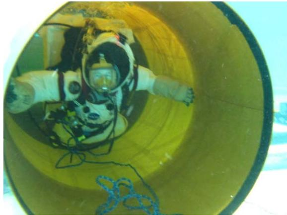
Figure 25. Test subject in MX-B egressing Dream Chaser in neutral buoyancy from aft hatch
