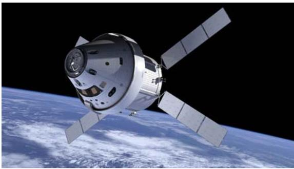
**Figure 1. Lockheed Orion spacecraft with initial ATV-derived service module**
