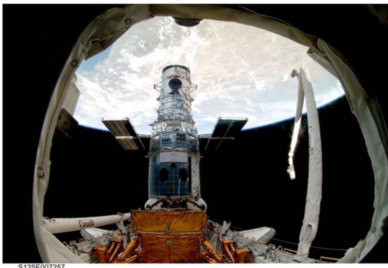
Figure 8. Hubble Space Telescope in orbiter payload bay for EVA servicing
