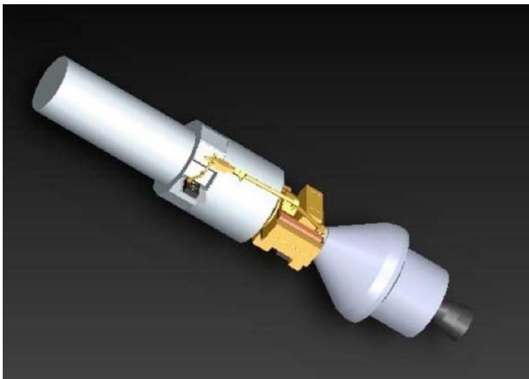
Figure 9. Concept for SM-4 servicing performed from Orion spacecraft with dexterous robotic assistance
