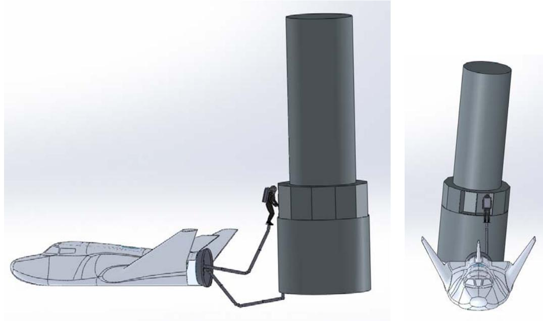
**Figure 21. Dual manipulator HST servicing concept for SNC Dream Chaser** **Figure 22. Dual manipulator HST servicing concept for SNC Dream Chaser**
