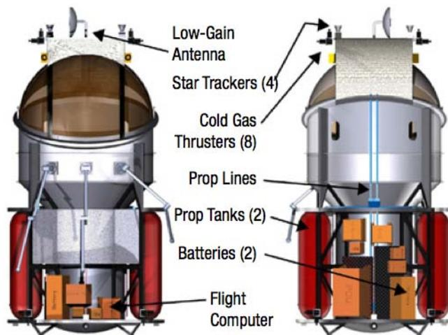
Figure 26. FlexCraft orbital utility vehicle concept<sup>4</sup>
