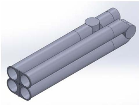
Figure 14. Folding 7DOF manipulator concept for SNC Dream Chaser (stowed)
