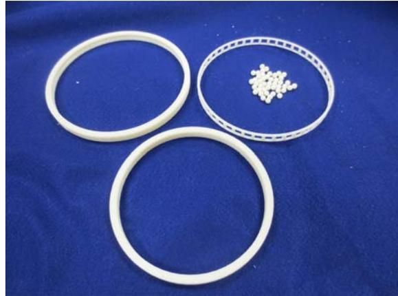
Figure 11. Components of 3D printed bearing disassembled
