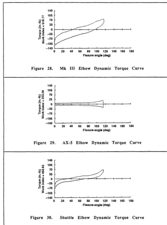
Figure 9. Torques in elbow motion for suits under test<sup>3</sup>
