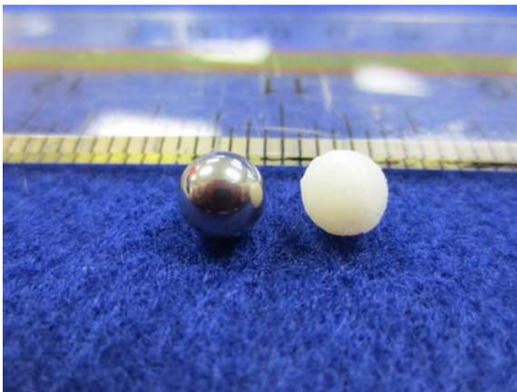
Figure 12. Prototype bearing balls: in-place fabricated (right); commercial stainless steel balls (left)
