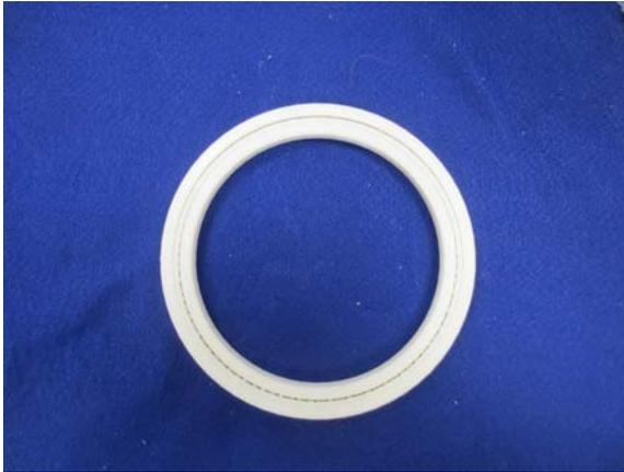
Figure 10. Test bearing manufactured assembled by fused deposition
