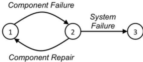
**Figure 2. SMP diagram for a notional single-string system with limited survival time after component failure, showing transitions between the nominal state (1), an offline but recoverable state (2), and a state in which the system has reached an unrecoverable failed state (3).<sup>8</sup>**
