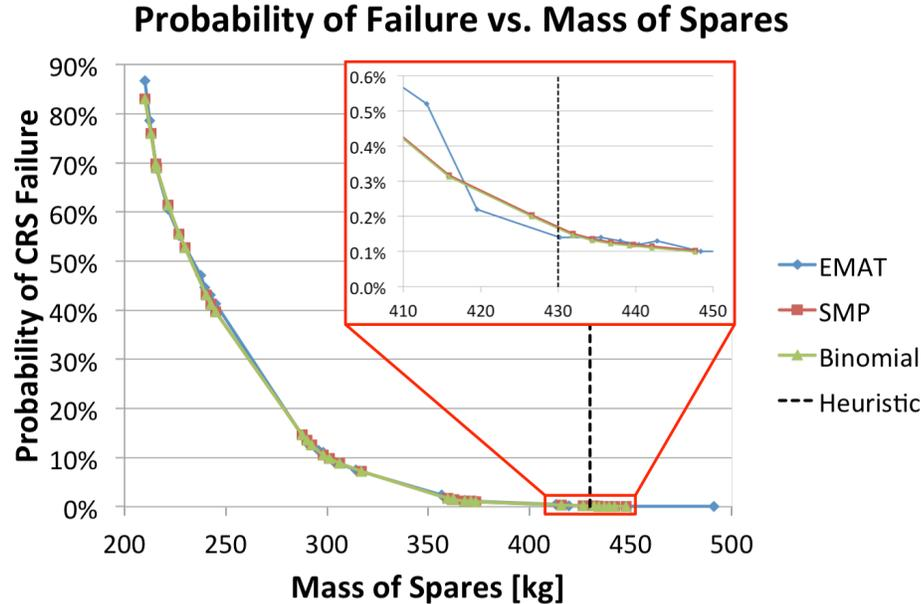
**Figure 4. Probability of CRS failure as a function of spares mass, as calculated using EMAT, SMP, and the binomial method. The mass value estimated by the heuristic method is also shown. The red inset figure shows a detailed view of the region immediately around the heuristic mass estimate. The mass of spares includes spare components for CDRA and the LiOH scrubber as well as the mass of a 30-day contingency LiOH supply.**
