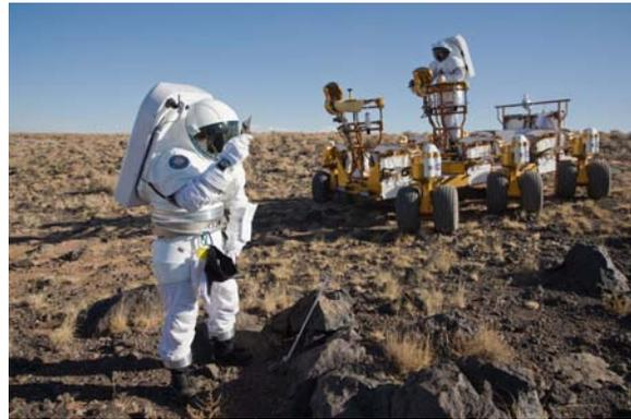
Figure 5. Unpressurized full-spectrum suit used with Chariot unpressurized rover
