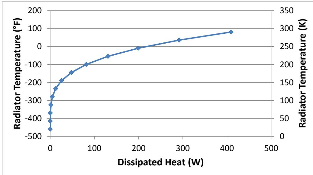
Figure 3. Dissipated Heat as a Function of Radiator Temperature for a 1m<sup>2</sup> Black Radiator.
