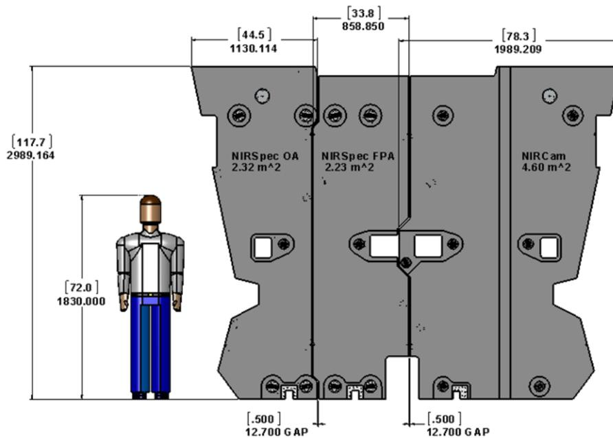
Figure 4. Dimensioned CAD Image of FIR. Dimensions in millimeters [inches].
