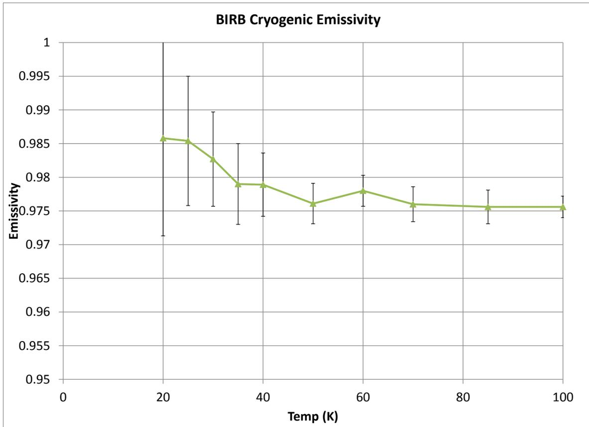
**Figure 7 BIRB™ Emissivity Performance as a Function of Temperature.**
