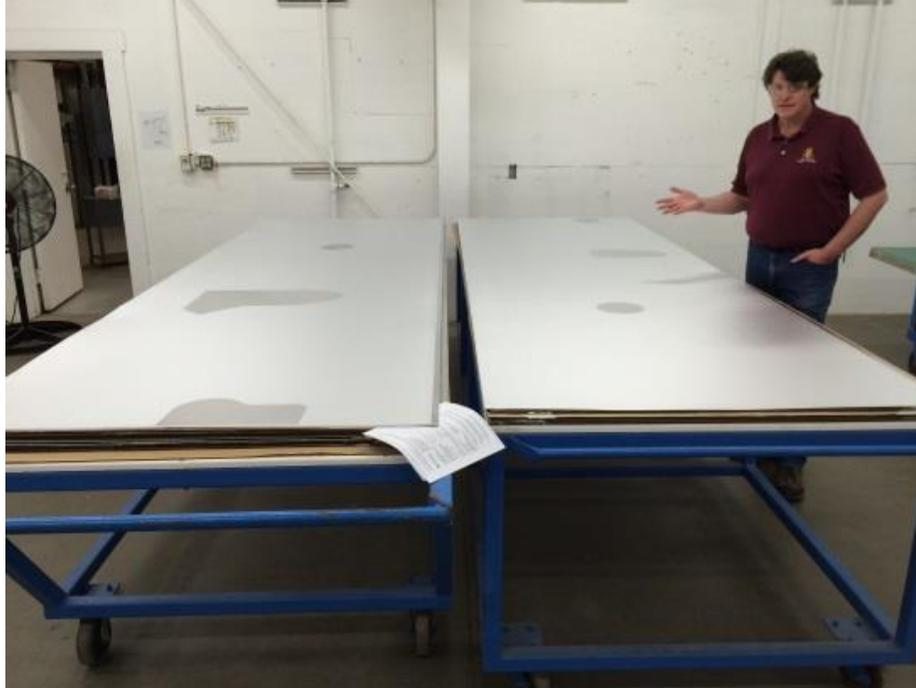
**Figure 6 FIR Facesheets After Milling Operations.**
