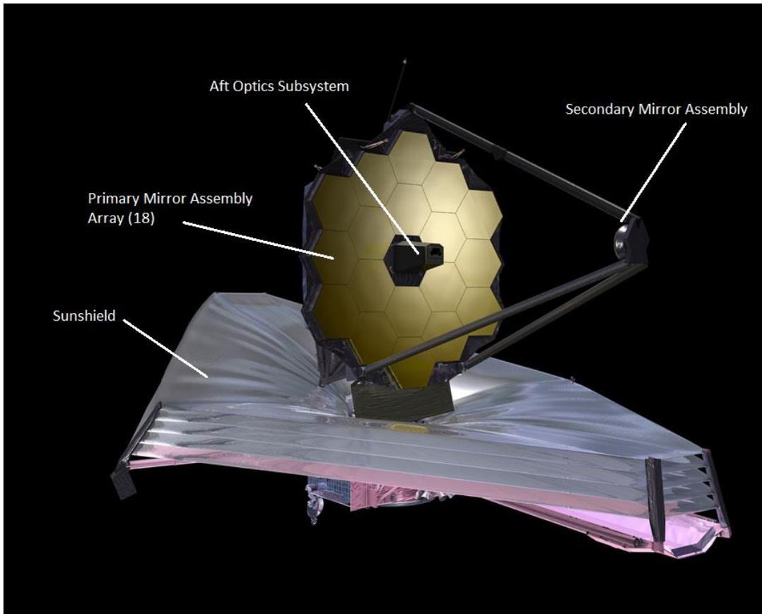
**Figure 1. James Webb Space Telescope with Sunshield and Optical Elements Labeled.**
