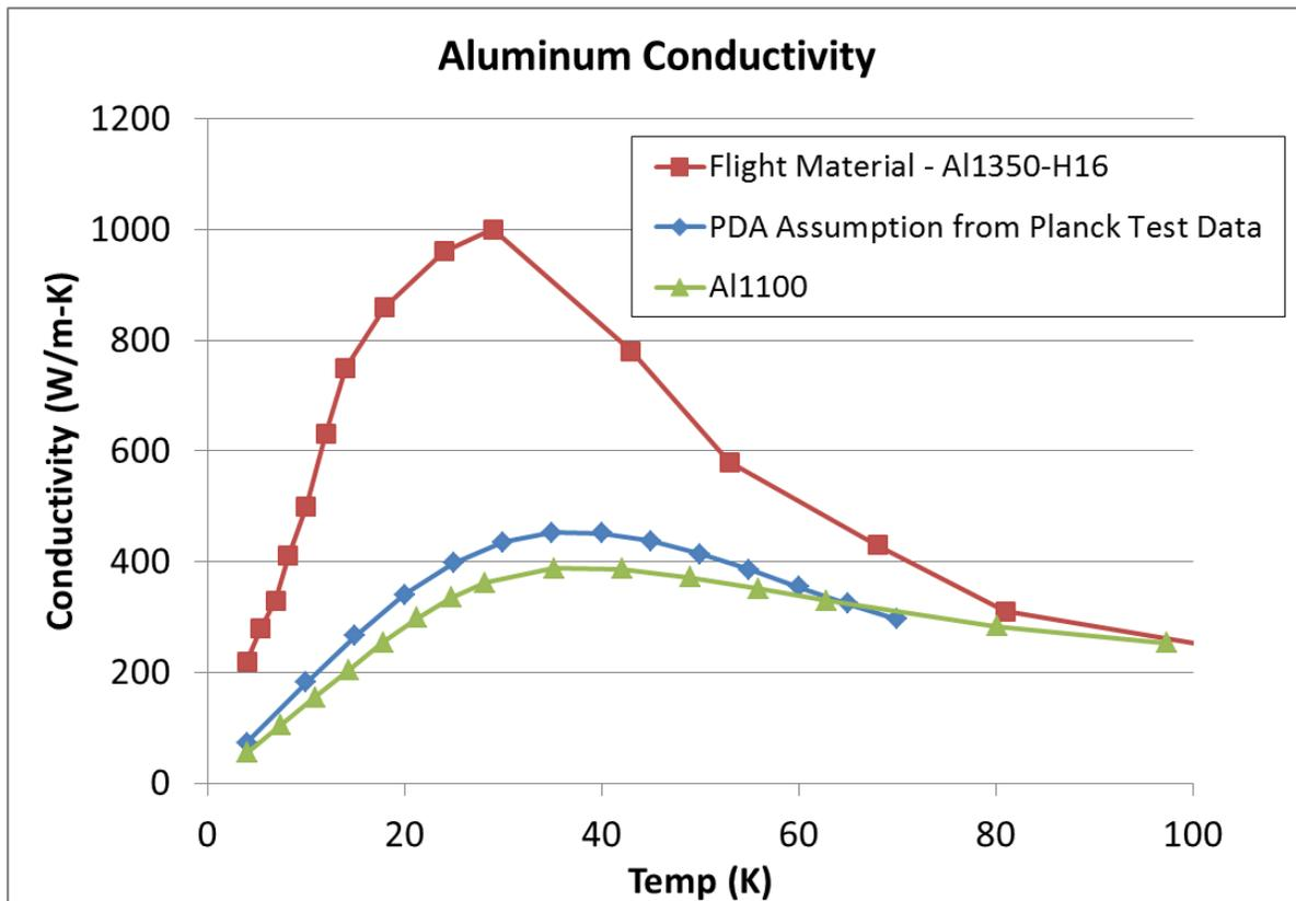
Figure 5 Comparison of the Flight Aluminum (1350) Conductivity to Traditional Al1100.
