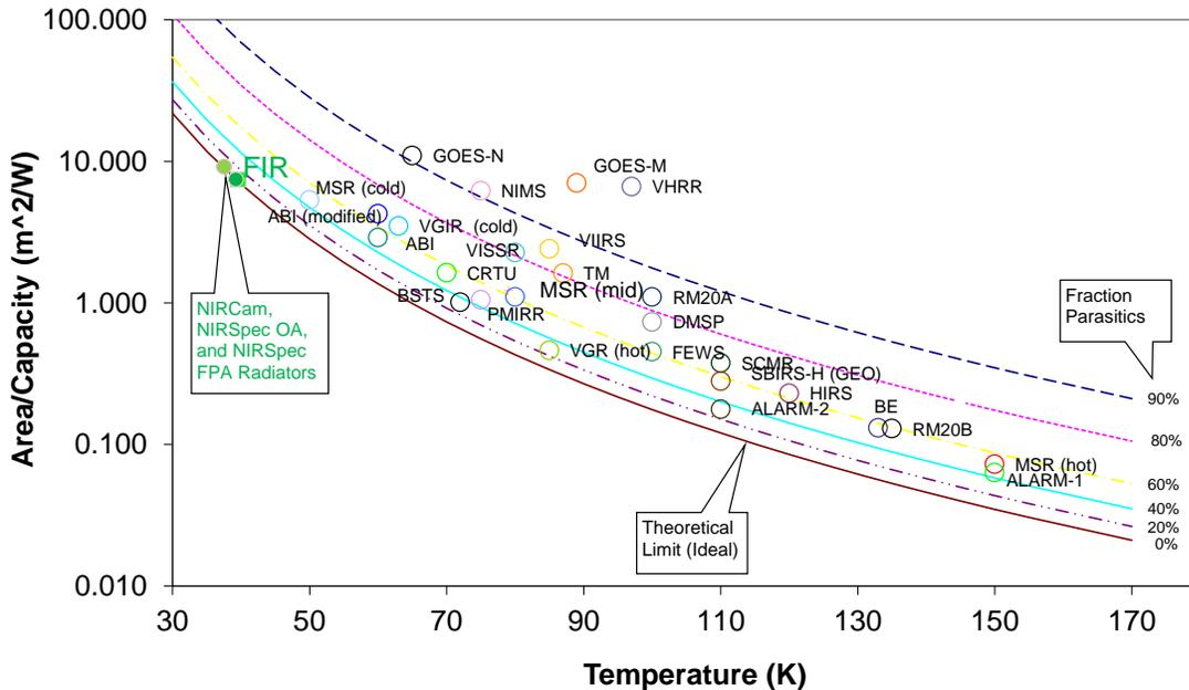
Figure 11 Performance of Radiant Coolers with FIR Included. Graph adapted from the Satellite Thermal Control Handbook, Vol II: Cryogenics, Figure 6.13<sup>5</sup>.
