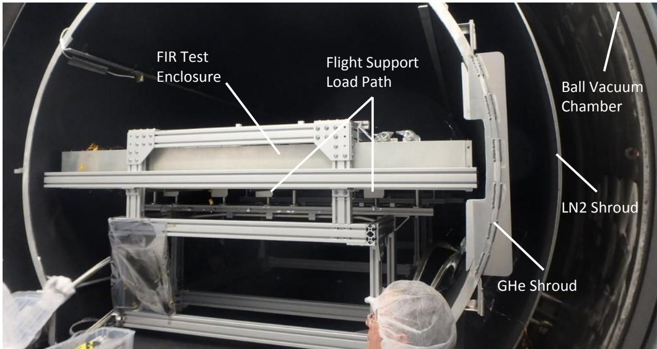
Figure 10 The FIR Thermal Test Environment.
