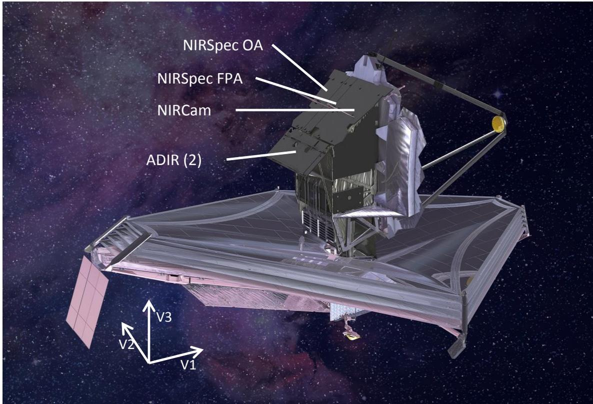
Figure 2. James Webb Telescope with the 5 Cryogenic Radiators, Labeled.
