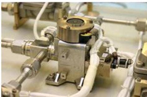
**Figure 10 Motorized 3-Way Valve (MPFL)**
