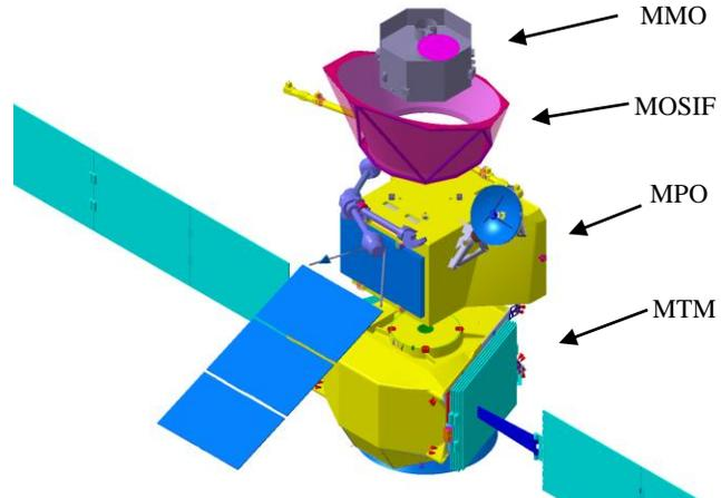
**Figure 1. Mercury Composite Spacecraft composed of MTM, MPO and MMO inside its sunshade MOSIF.**
