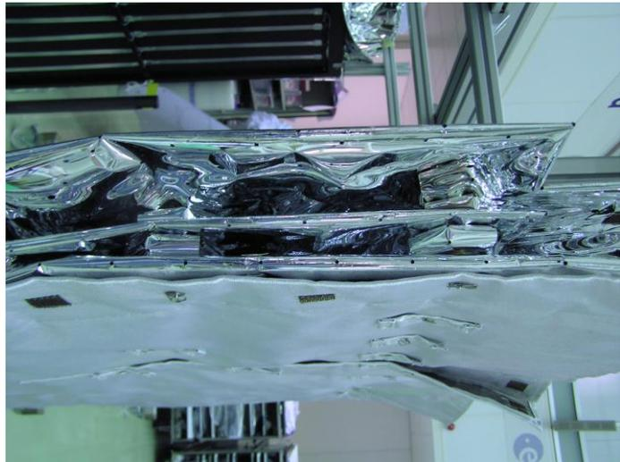
**Figure 5. Flight MLI Configuration.**
