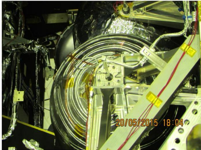
Figure 6. Wire Heaters layout on tank -Y.
