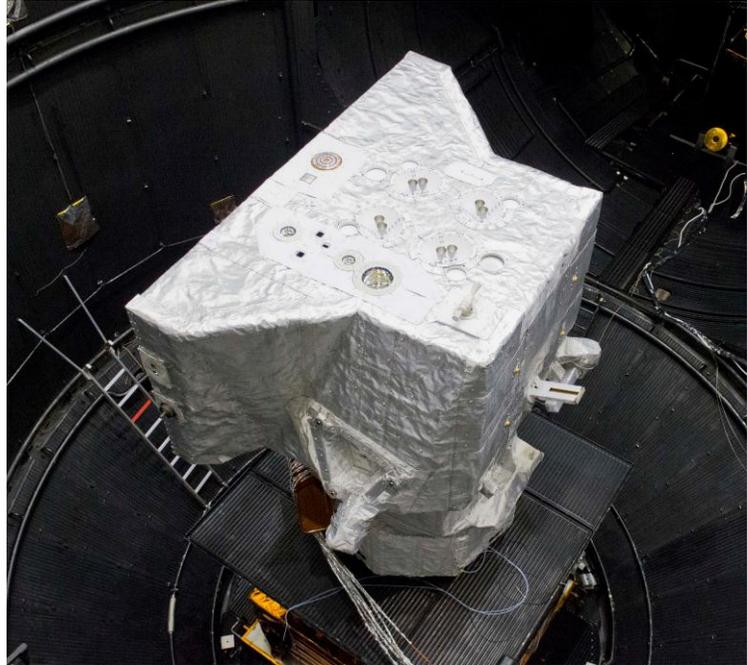
**Figure 2. MPO inside the LSS chamber.**
