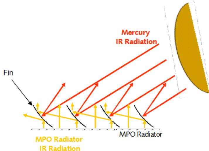
Figure 4. Radiator Reflector concept.
