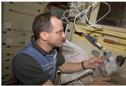
Figure 3 - SVO-ZV water dispenser. Collection of water sample from SVO-ZV by Donald Pettit (NASA/JSC Photo #ISS006E08628)
