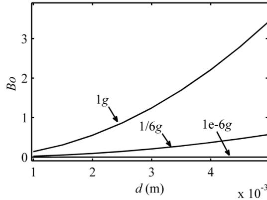
**Figure 4. Bond number variation with characteristic parameter of feed water gap**
