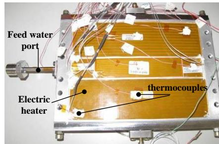
Figure 6. The test module of sublimator
