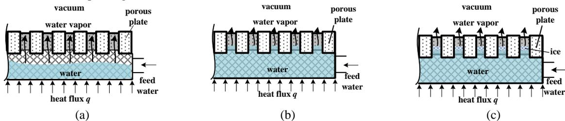
Figure 1. Water sublimator startup processes
