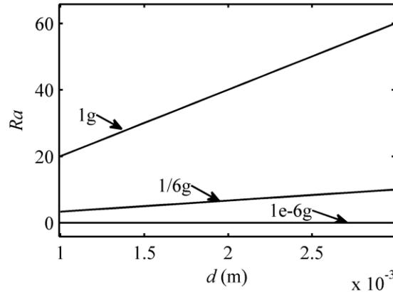
**Figure 5. Rayleigh number variation with characteristic parameter of feed water gap**
