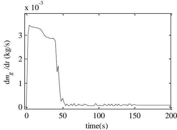
**Figure 2. Feed water mass flow rate in the startup process of sublimator**
