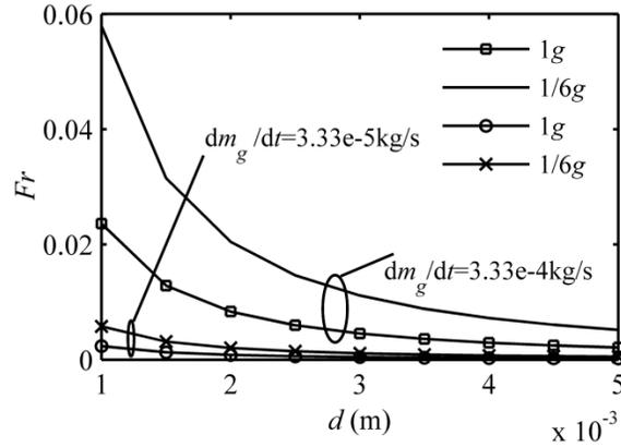
**Figure 3. Froude number variation with characteristic parameter of feed water gap**
