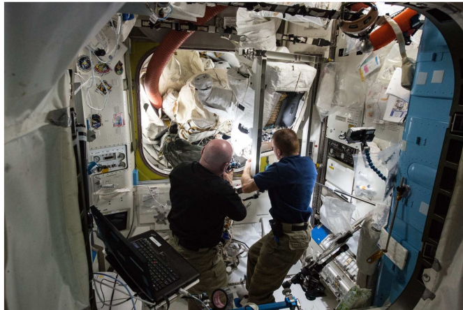
Figure 5 – Astronauts Scott Kelly & Terry Virts changing out the EMU Fan/Pump/Separator during Expedition 26.
