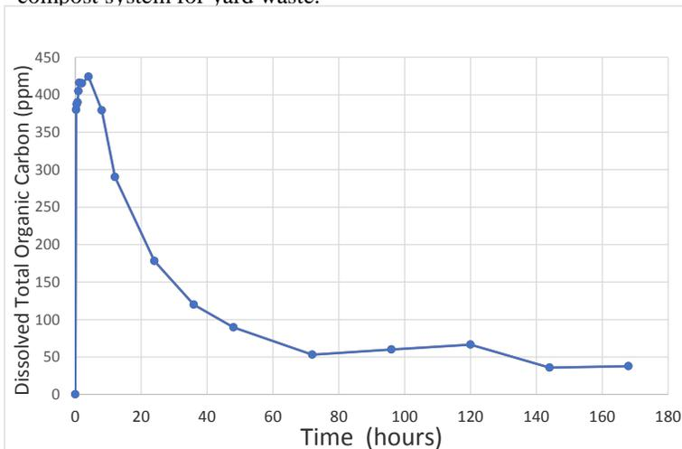
**Figure 5.** TOC concentration in a stirred flask reactor following addition of 25 g L<sup>-1</sup> of dried ground tomato biomass (inedible leaves and stems), and a microbial inoculum from a home yard-waste compost pile. Solution volume for the reactor was 2 L.
