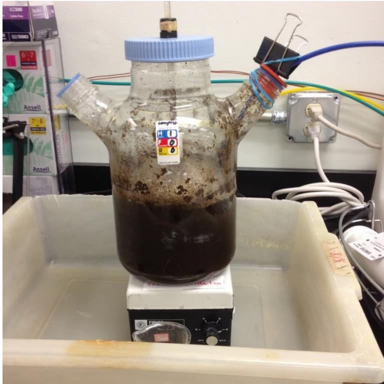
**Figure 4.** Stirred-flask reactor used to track TOC concentration degradation over time. Testing used a working volume of 2 L of solution to which 50 g of dried ground tomato biomass was added, along with a microbial inoculum originally obtained from a home compost system for yard waste.
