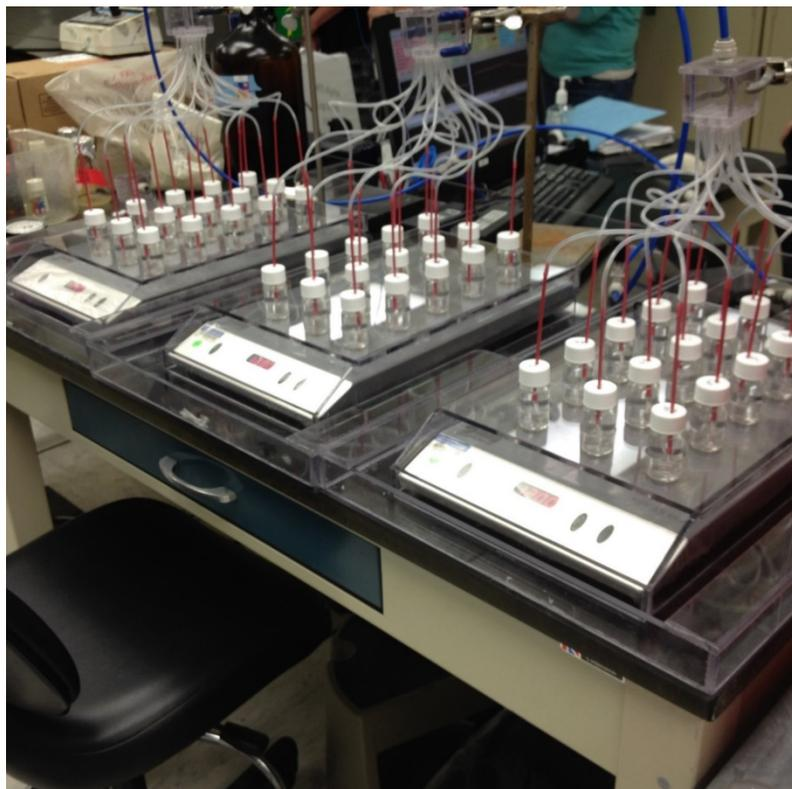
**Figure 1.** Vial minireactors, referred to as VOA (volatile organic analysis) vials, used for various treatments of inedible plant biomass. For some treatments, vials were continuously aerated at 60 mL/min and volumes were adjusted as needed to offset evaporation. The small vials allowed simultaneous testing of multiple treatments.
