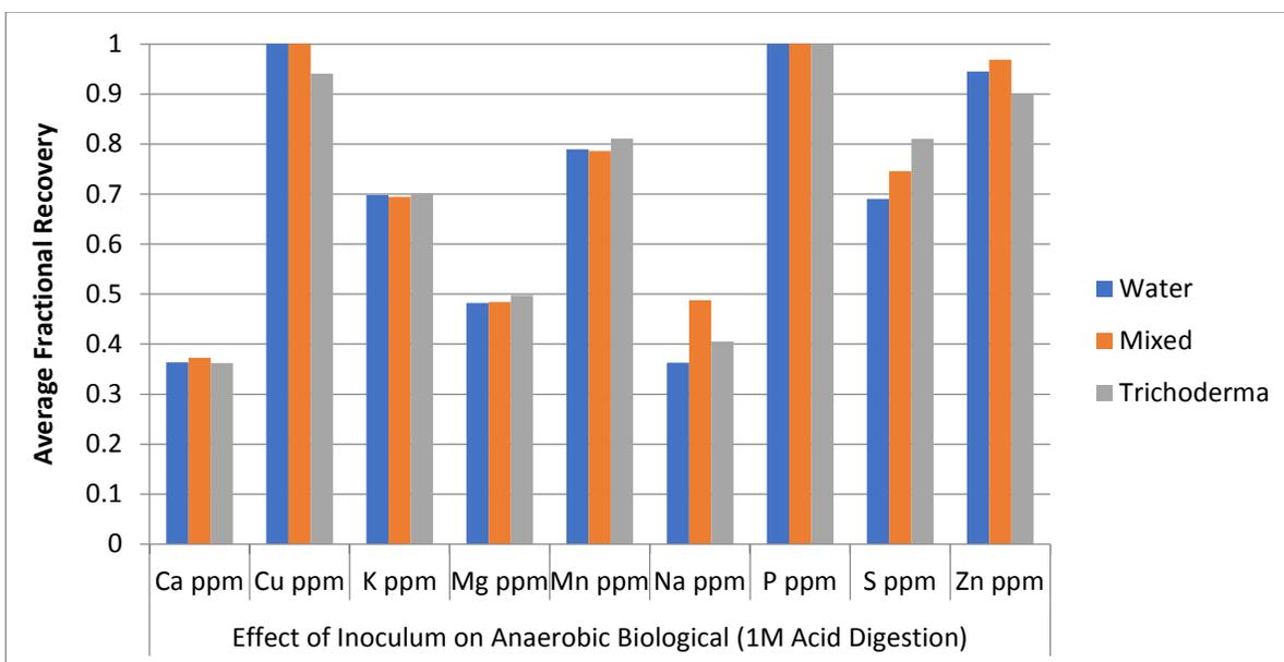
**Figure 3.** Effect of biological inocula on nutrient recovery from dried inedible pepper biomass followed by a 0.1 M HCl acid digestion. Anaerobic refers to the use of nonaerated vials.
