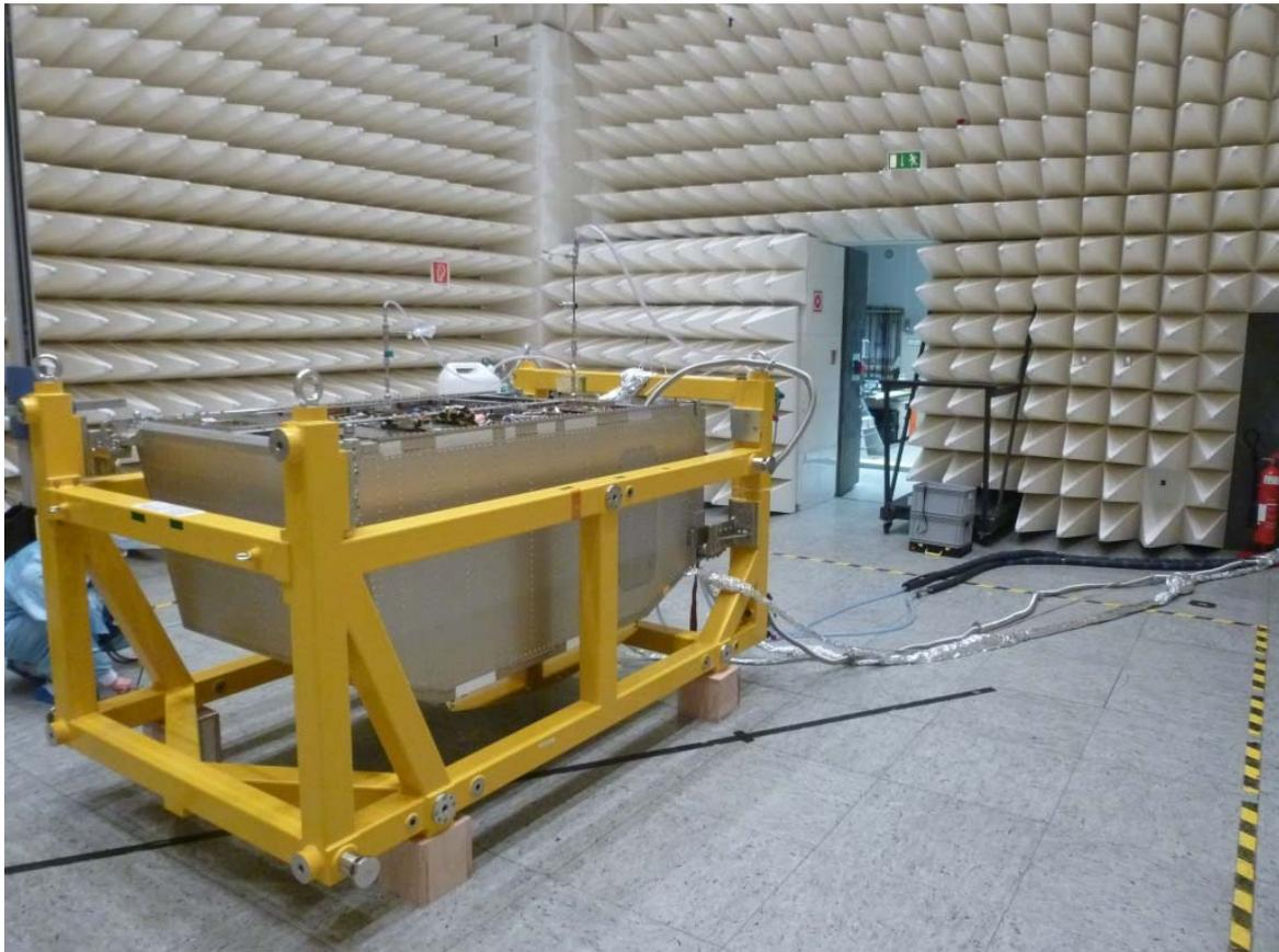
**Figure 15: Rack Level EMC Testing**
