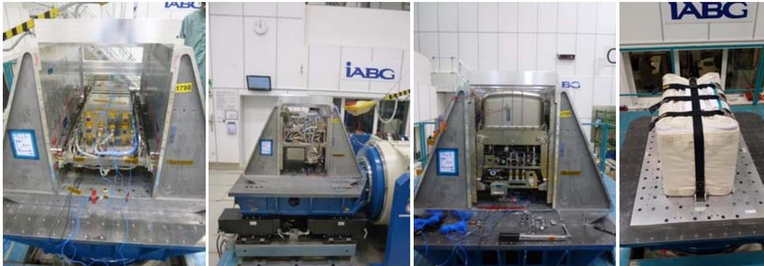
**Figure 14: Vibration Testing (Drawer Level - integr. Launch Config. vs. CTB Level - separate Launch Items)**
