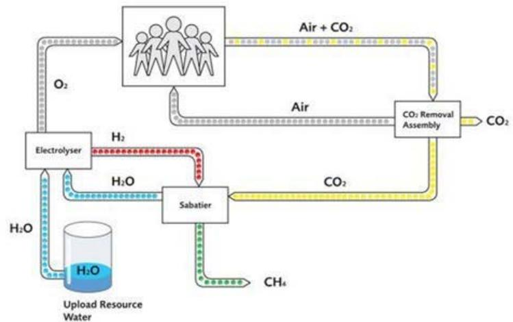
Figure 1: ACLS Closed Loop Schematic
