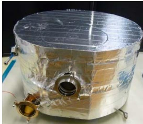
Figure 6: FM CO<sub>2</sub> Adsorber Bed
