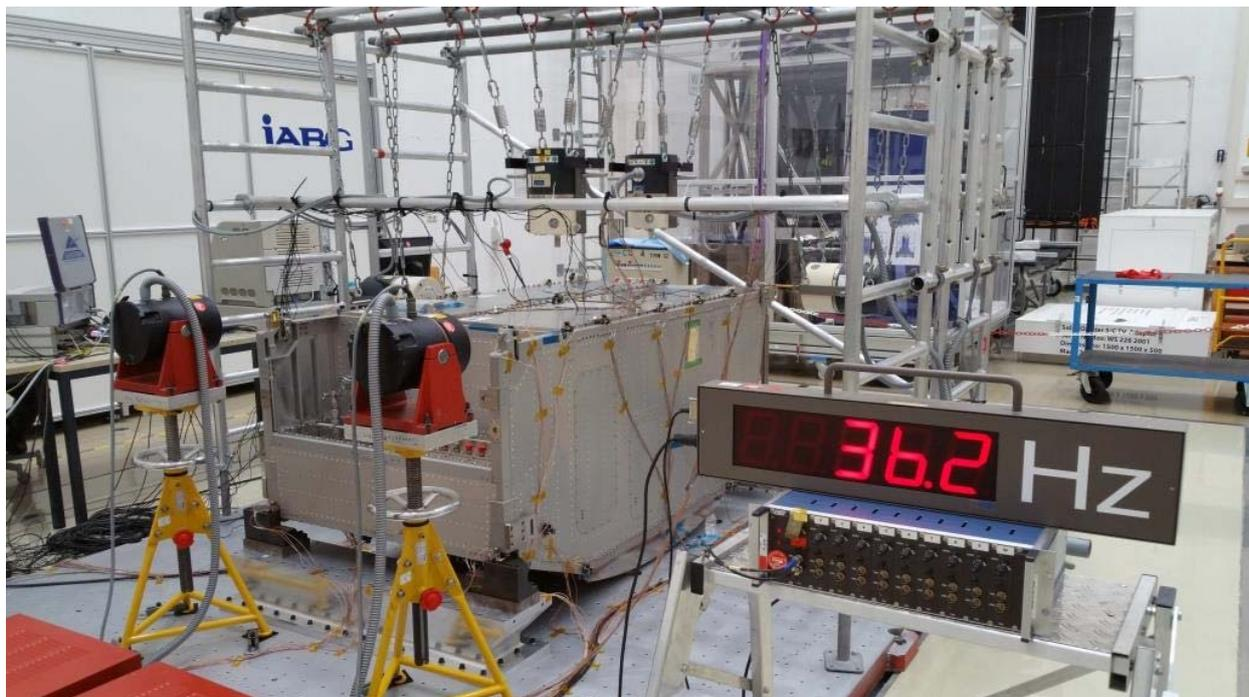
**Figure 13: Rack level Modal Survey Testing (MST)**
