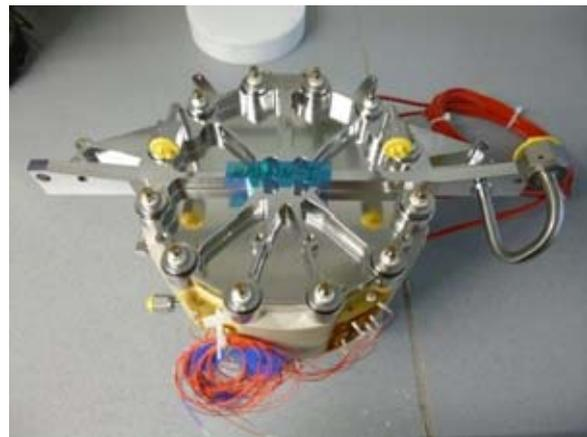
Figure 11: KOH Filter (Top) and Electrolyser Stack (Bottom)
