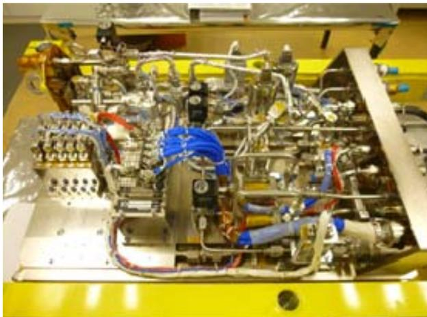
Figure 5: FM Drawer 1 with CO<sub>2</sub> Management Section
