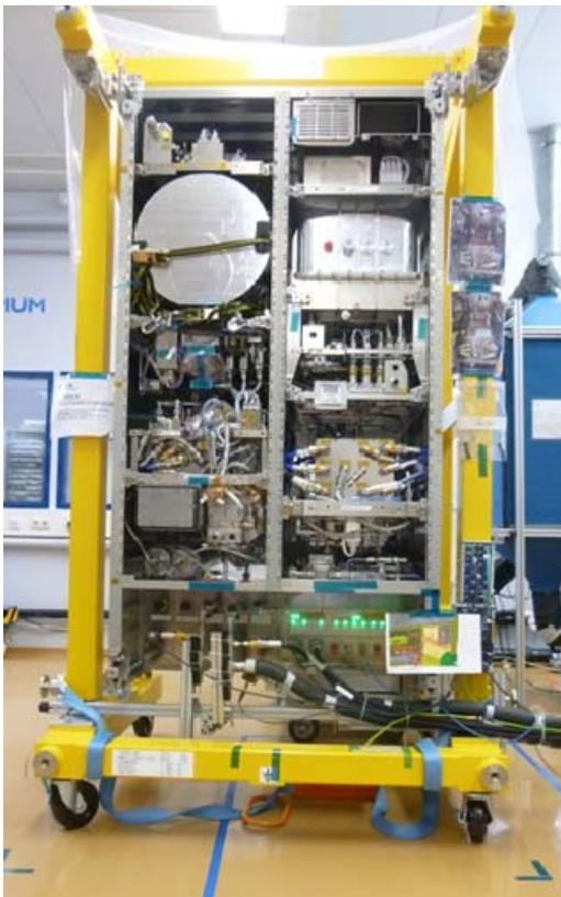
Figure 3: FM Rack with all integrated Drawers (w/o closure panels)
