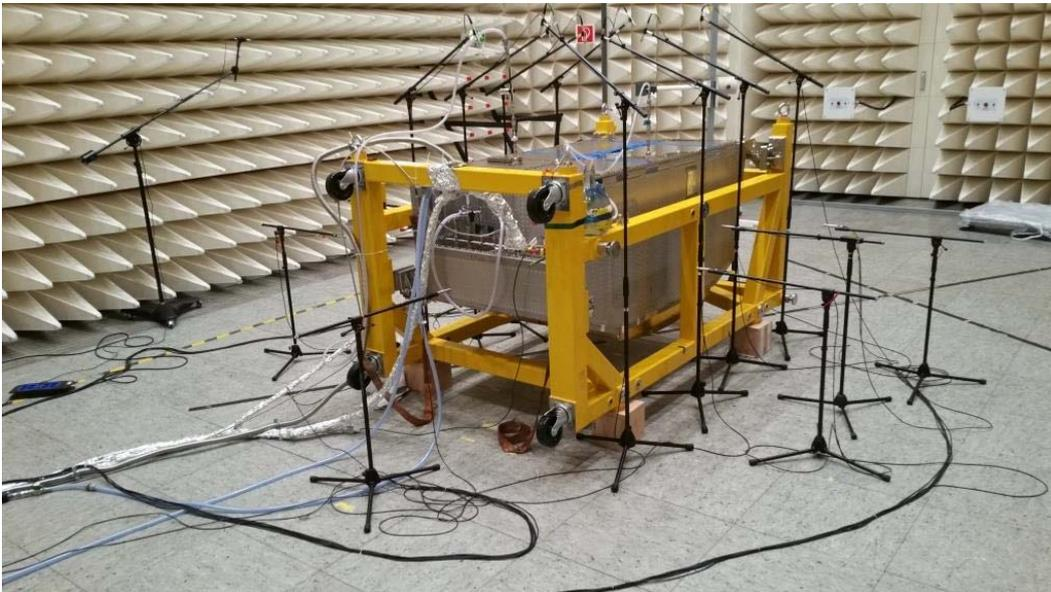
**Figure 16: Rack Level Audible Noise Testing**
