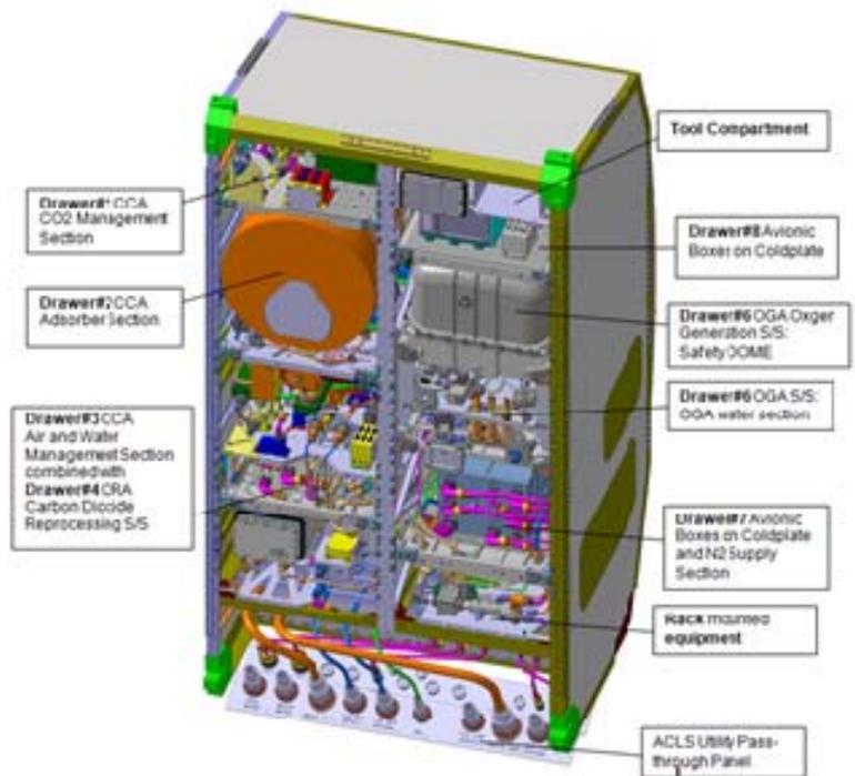
Figure 4: ACLS front view w/o Front Panels
