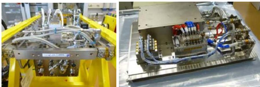
Figure 12: Avionics Drawer 7 incl.  $N_2$  supply Section (left) and Avionics Drawer 8 (right)
