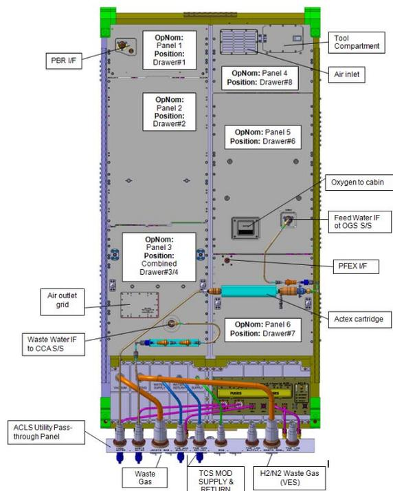
Figure 2: ACLS Interfaces and Front Panel Equipment
