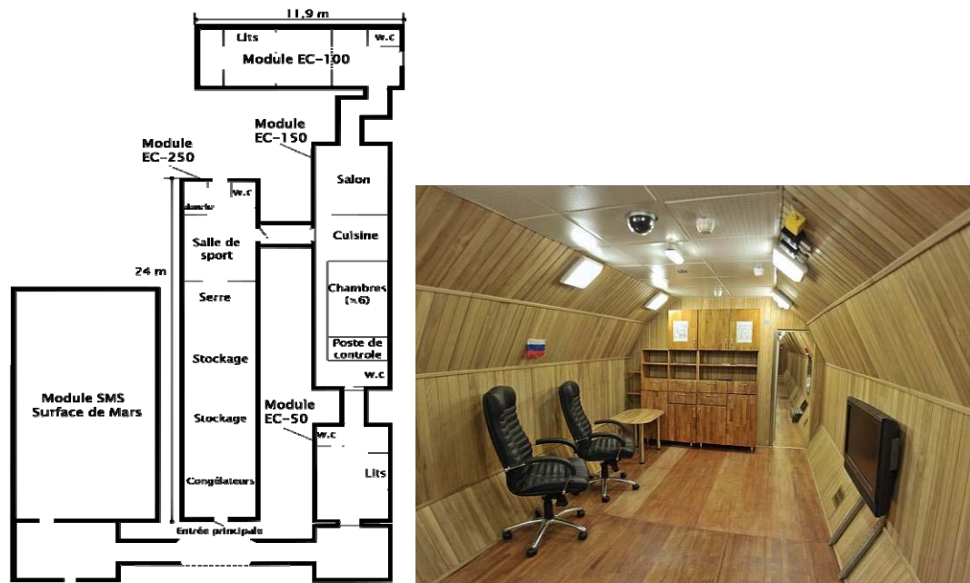
Figure 6. The Mars500 Isolation Facility Plan of the experimental complex. Module Simulator of Martian surface, Module EC-50 (Simulator of the landing Martian ship), Module EC-150 (Habitable module with 6 individual compartments, community room, main console, kitchen, lavatory), Module EC-250 (Utility module with gym, greenhouse, storage for resources, fridge, thermal chamber, lavatory), Module EC-100 ( Medical module with habitable compartment, kitchen-dining-room, working places with medical equipment and lavatory). (Armael)
