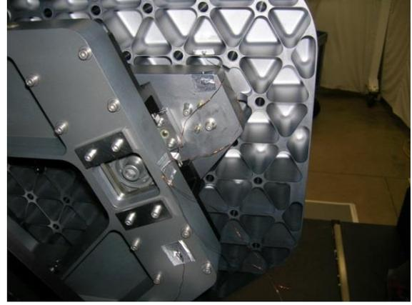
Figure 5. Light-weighting pockets in the back of the tertiary mirror substrate.
