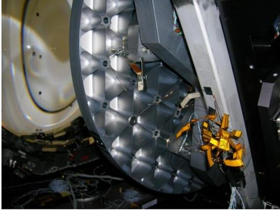
Figure 4. Light-weighting pockets in the back of the secondary mirror substrate.
