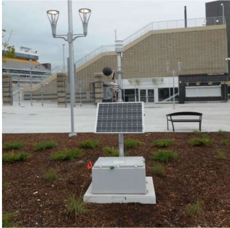
Figure 2.4. Hamilton Soccer Centre mesonet station used to monitor environmental conditions during the Games' soccer events. Source: Environment Canada.
