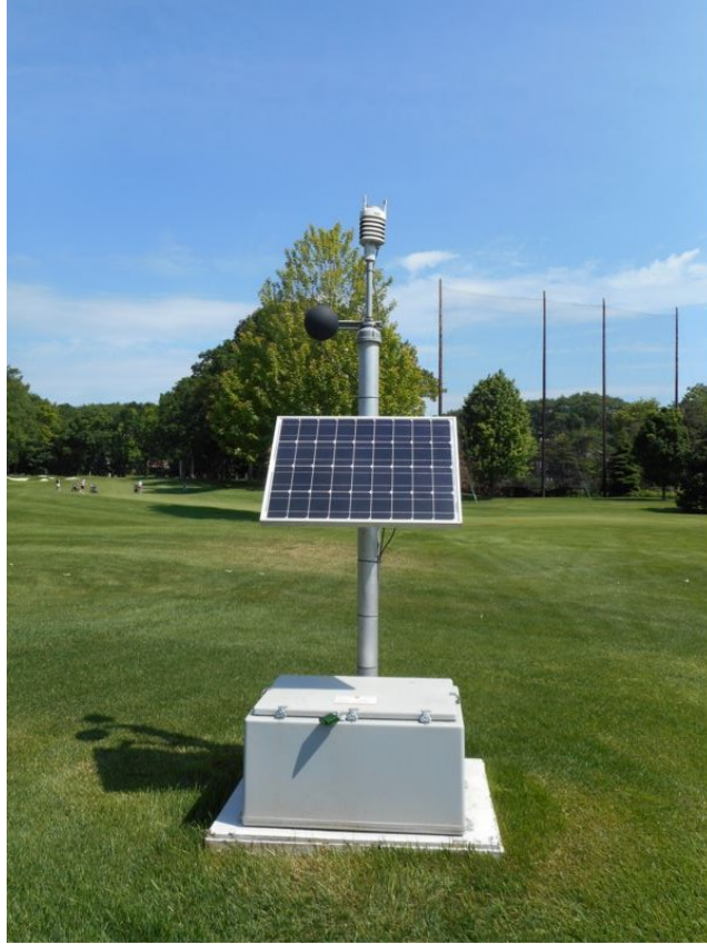
Figure 2.2. General structure of one of the 43 temporarily installed compact mesonet stations used to monitor environmental conditions during the Games. Source: Environment Canada.
