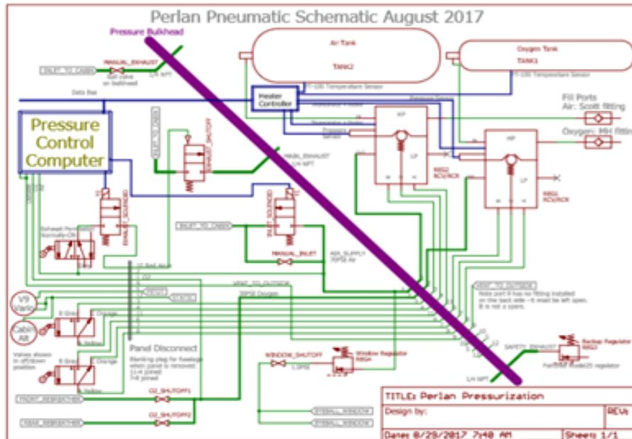
Figure 4. Perlan II Pressurization Schematic
