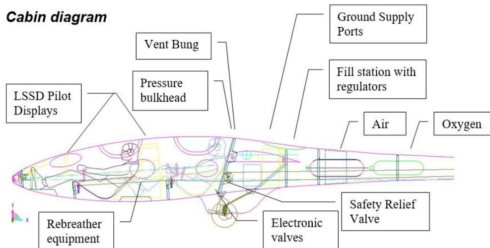
Figure 3. Perlan II Cabin Diagram
