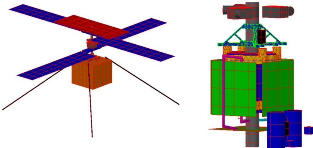
Figure 3. Images of the helicopter thermal model from the external (left) and internal (right) views.
