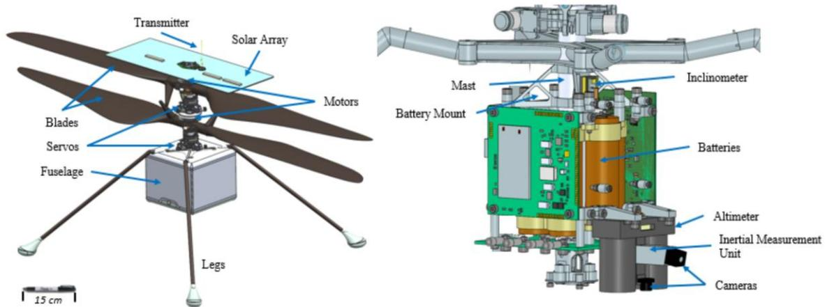
**Figure 1. Model images of the helicopter concept. The left image shows the exterior components with a marker shown for scale. The right image shows the interior components, including the printed wiring boards, cameras, sensors, and batteries (one of the boards is hidden so the batteries are visible).**
