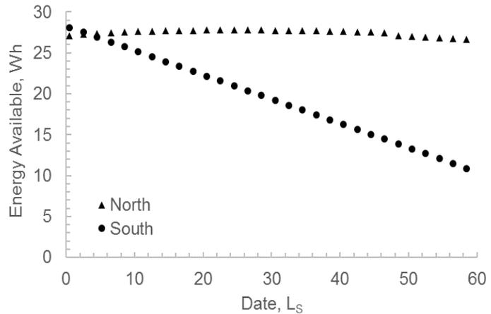
Figure 2. Maximum energy available in the batteries as a function of mission time.
