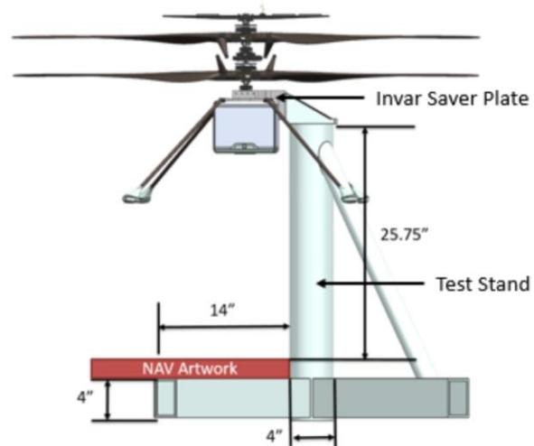
Figure 5. Test setup for helicopter. The test stand is a welded aluminum frame with an invar saver plate that interfaces with the helicopter mast. An artwork pattern below the helicopter provides a target for the nadir camera.
