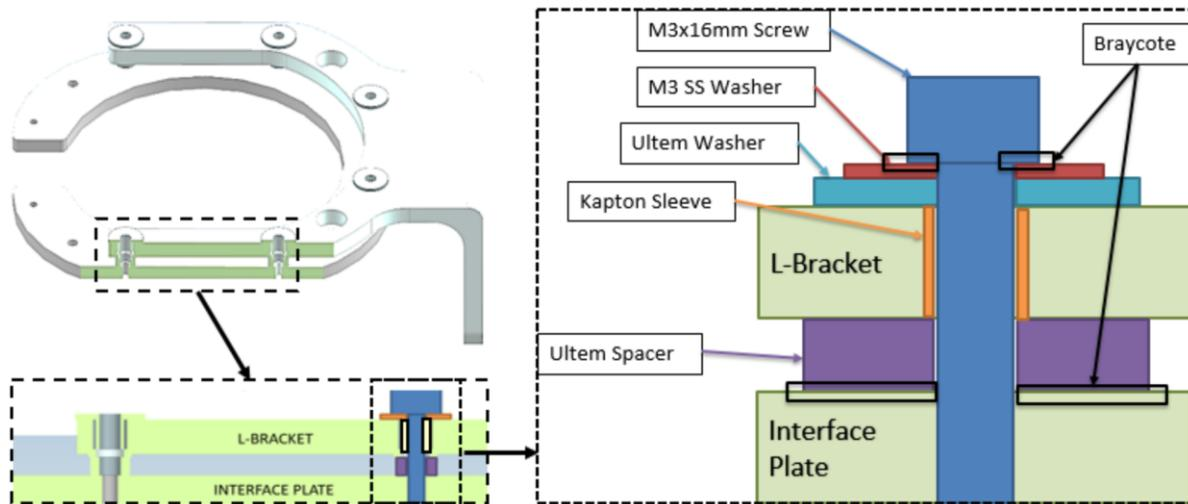
**Figure 6. Thermal isolation scheme for the helicopter. The upper left image shows the L-bracket and interface plate where they would meet with the helicopter mast. The lower left image shows a cross section view of the interface with the middle spacer plate layer included. The right image shows the thermal isolation scheme at the bolted interfaces.**
