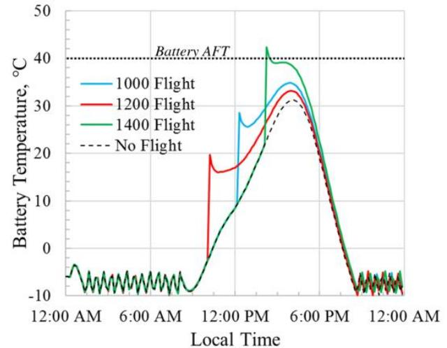
Figure 4. Parametric variation of the time of flight at the northern landing site.
