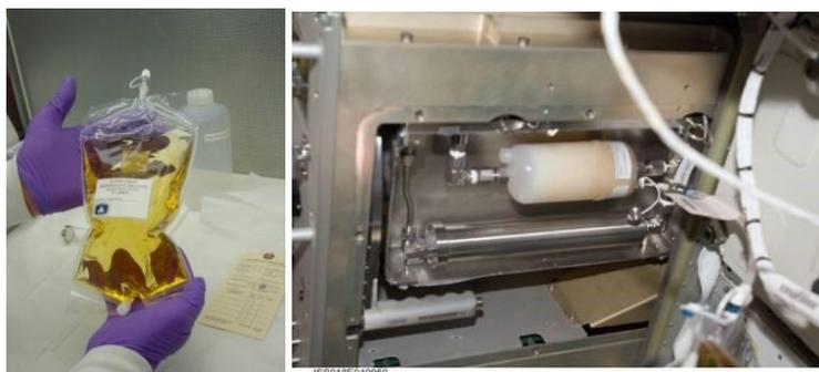
Figure 5. PWD shock kit bag (left) and shock kit in use (right).
