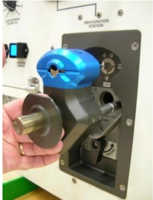
**Figure 3. Rehydration Station with Beverage Adapter Assembly.**
