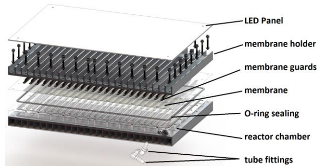
Figure 7: The components of the µgPBR.
