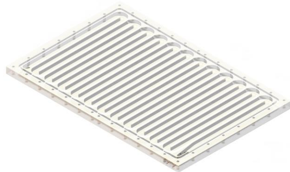
Figure 8: Reactor chamber with meander like flow path.
