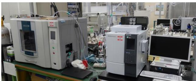
Figure 8 Microwave methane decomposing test equipment
