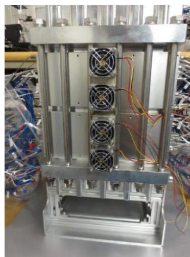
Figure 6. Reaction vessel of full-scale prototype
