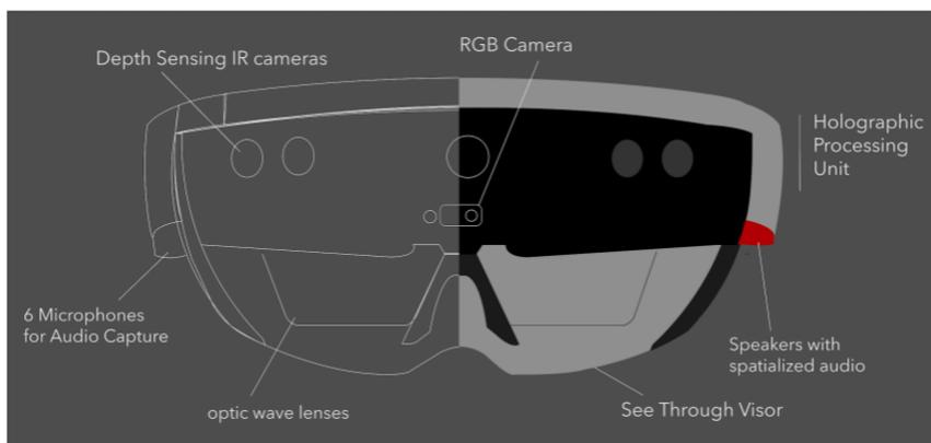
**Figure 4. Microsoft HoloLens hardware front view, with components, highlighted**
