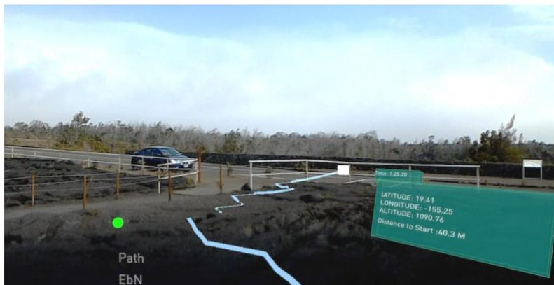
**Figure 8. First person view of UI. Include, path, waypoint, and status display**
