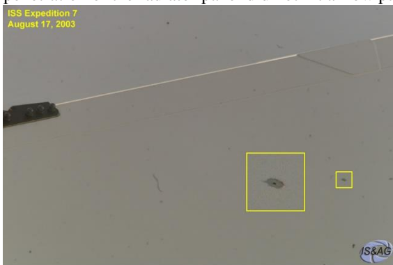
Figure 6 – MMOD damage to an ISS radiator panel
