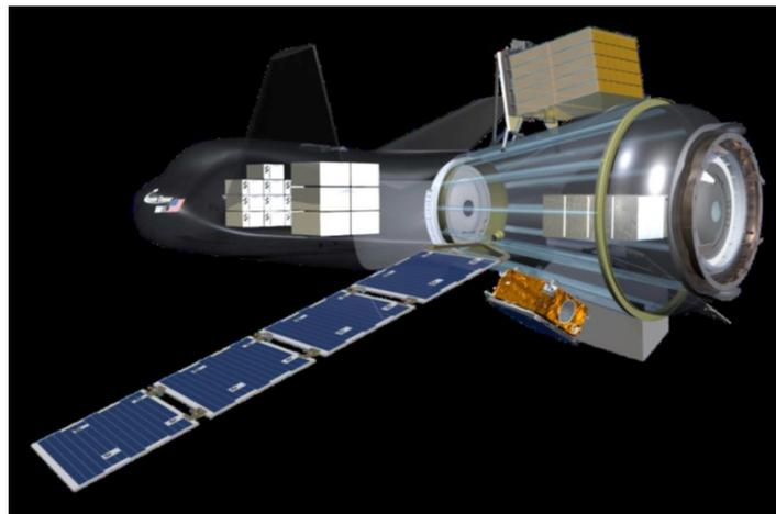
**Figure 6. Dream Chaser uncrewed configuration showing vehicle internal storage and detachable cargo module structure with external payload mounts and deployment mechanisms.**
