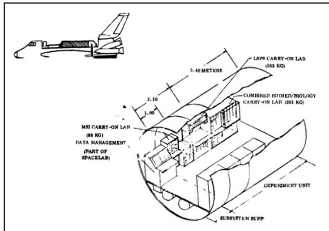
Figure 1. NASA Spacelab with Carry-on Lab concept<sup>3</sup> (credit-NASA).
