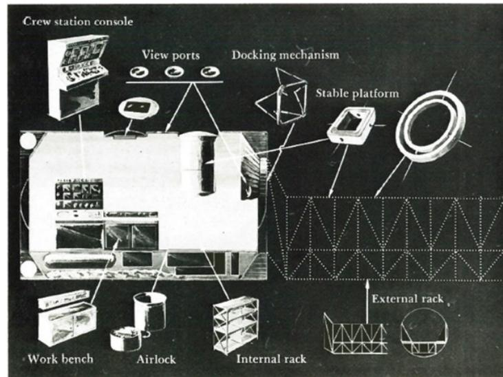
**Figure 3. Early concept of sortie module<sup>13</sup>. This was the precursor to Spacelab.**
