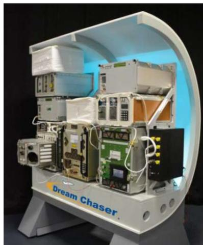
Figure 8. Early mockup of Dream Chaser sortie mission payload configuration based on use of middeck locker equivalent experiment carriers.
