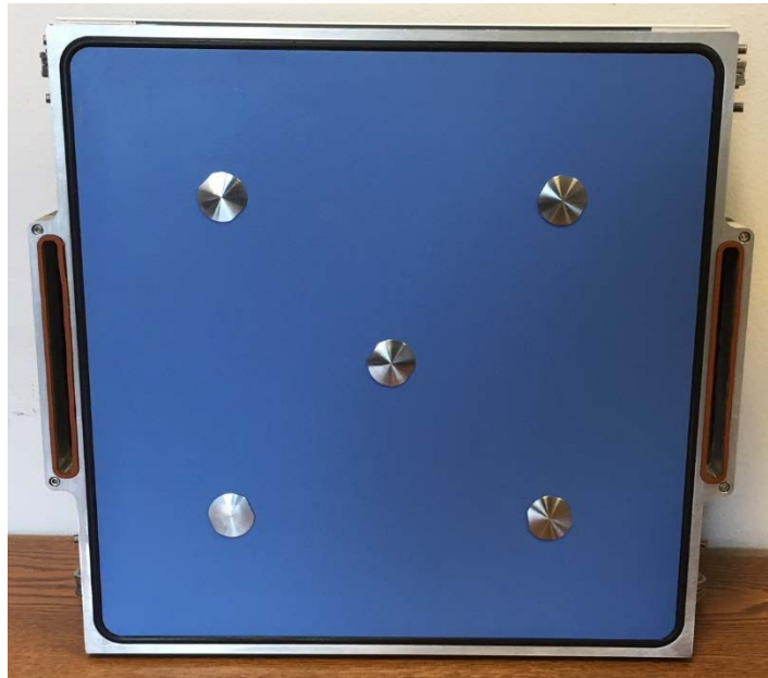
Figure 6. Chamber Door Interior Face with Vapor Ports
