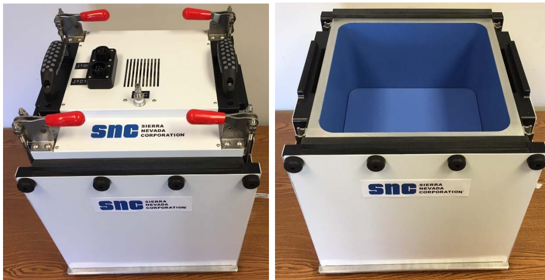
Figure 5. Processing Chamber with Door On (left) and Door Off (right)
