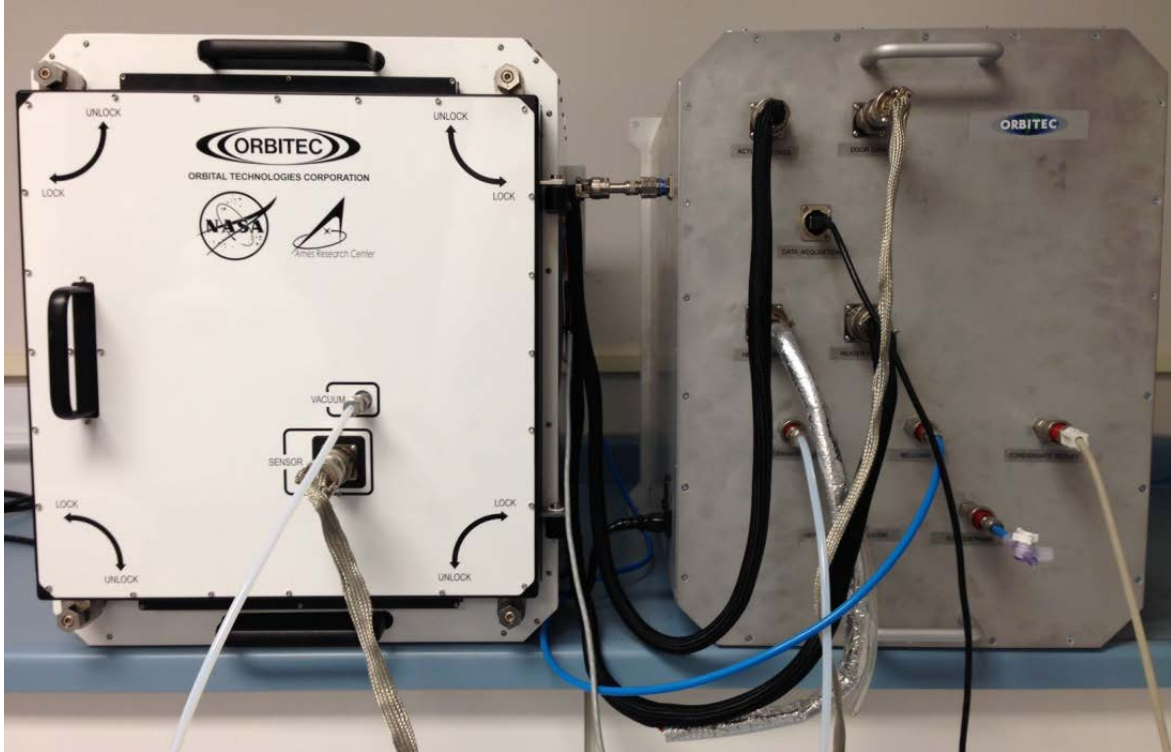
Figure 1. PMWC Prototype System: Processing Subsystem (Left); Support Equipment Subsystem (right)
