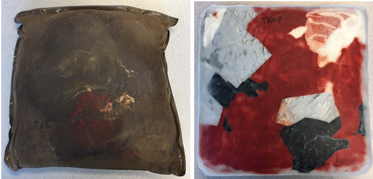
Figure 9. Resulting HMC Tile, showing Permeable Bag (left) and Plastic Trash Mix (right)
