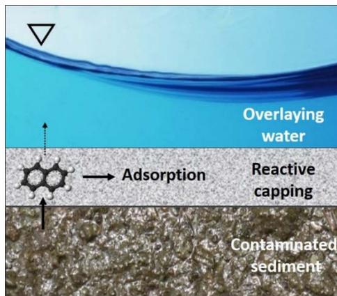
**Reactive capping** consists of one or more layers of adsorbent or reactive materials that sequester the contaminants; it decreases and delays the mass flux of contaminant to the overlaying water.
