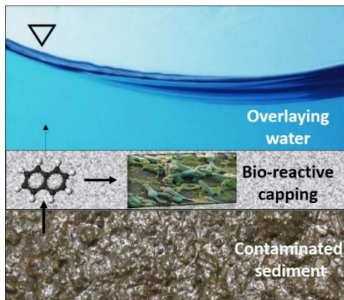
**Bio-reactive capping** consists of materials that sustain and promote the growth of native microbial communities able to degrade the contaminants; the mass flux to the overlaying water is delayed, and the pollutants are degraded within the capping system.
