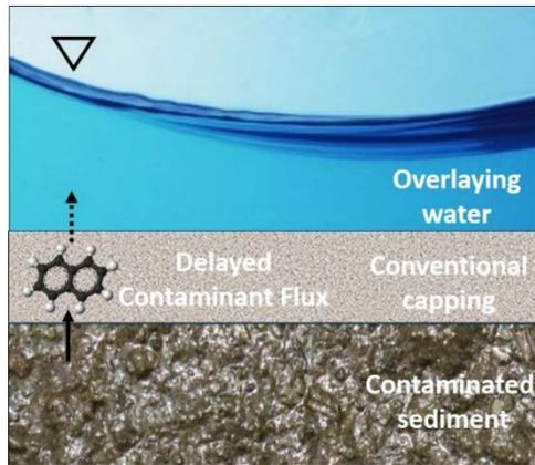
**Conventional capping** confines the contamination to the sediments and prevents erosion and resuspension; it delays the mass flux of contaminant to the overlaying water.
