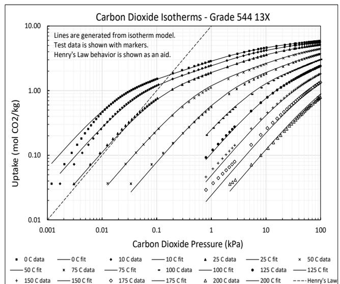
**Figure 2. Pure component CO<sub>2</sub> isotherms at temperatures from 0°C up to 200°C.<sup>6</sup>**
