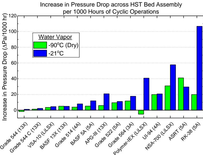
**Figure 1. Rate of pressure drop increase which correlates to sorbent dust generation in sub-scale beds under dry and humid conditions subjected to thermal cycling.<sup>5</sup>**
