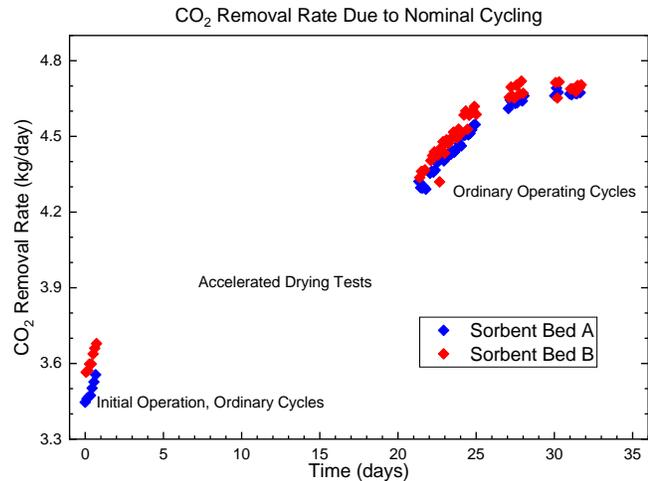
**Figure 8. Recovery of CO<sub>2</sub> removal performance after initial assembly which had exposed dry sorbent to ambient humidity. The CO<sub>2</sub> removal was impaired but increased after numerous operating cycles to a steady-state.**
