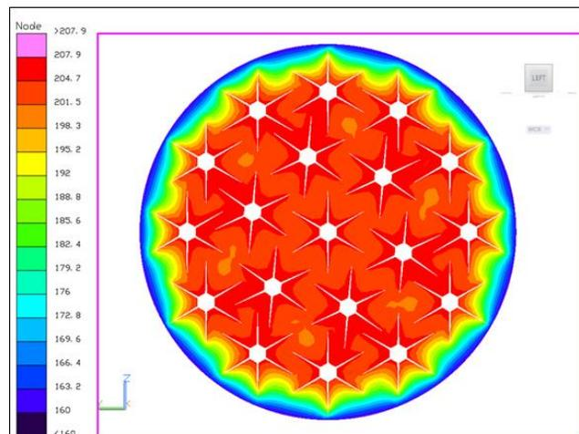
**Figure 4. Simulated temperature cross-section of a heating 4BCO<sub>2</sub> sorbent bed at the end of a half-cycle.<sup>18</sup>**
