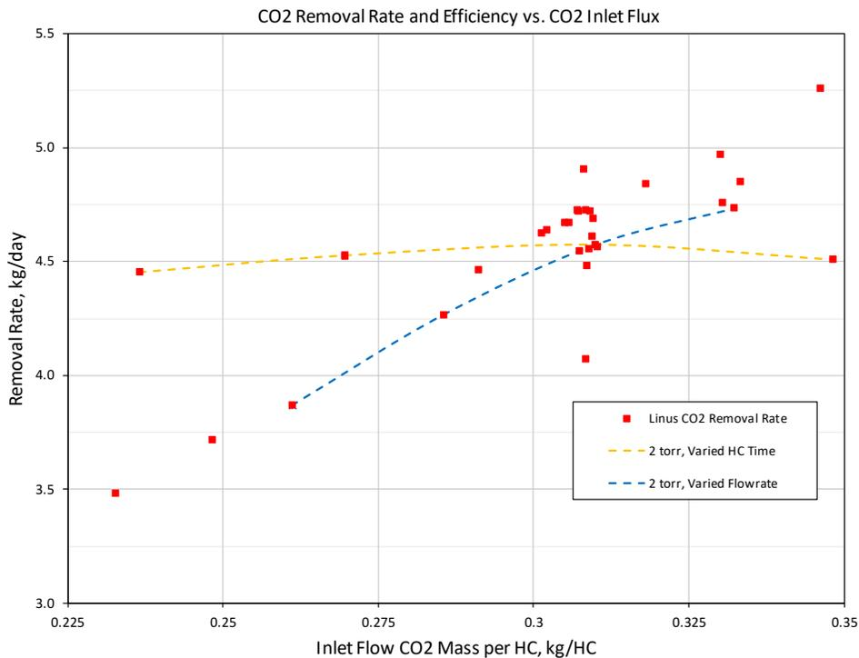
**Figure 11.** Performance map of Linus, the 4BCO<sub>2</sub> prototype. Blue and yellow dashed lines connect two selected test series where in each a single factor is varied.
