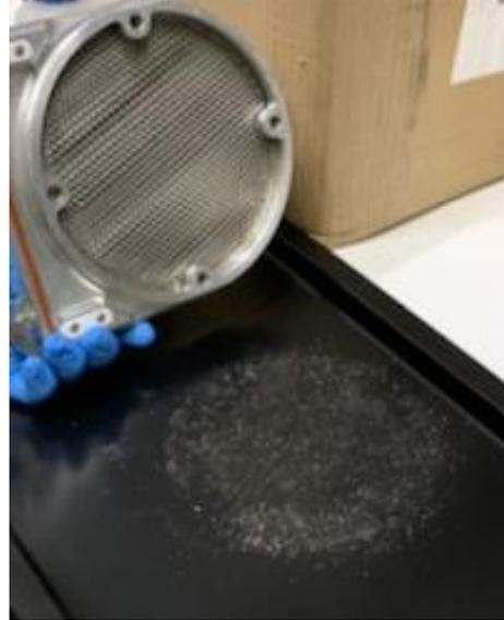
**Figure 10.** Dust recovered after 1000 hours of operation from Linus removable filters (also pictured). The black trays provide an enhanced visual contrast to view the dust.
