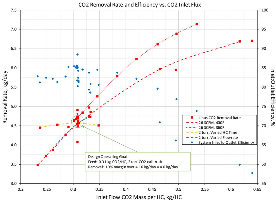
**Figure 13. Performance map of Linus, the 4BCO<sub>2</sub> prototype. Blue and yellow dashed lines connect two selected test series where in each a single factor is varied. Red dashed lines show two similar test series where the heater setpoint was set to 360°F and 400°F.**
