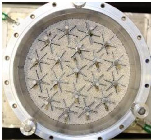
**Figure 6. Partially filled sorbent bed for the ‘Linus’ prototype 4BCO2 system.**
