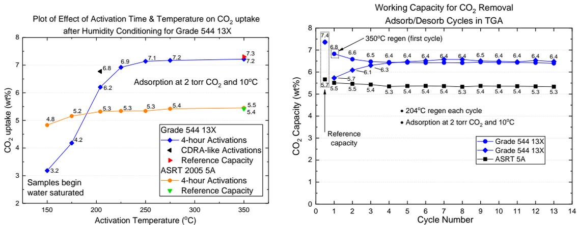
**Figure 3. Effect of activation temperature on sorbent performance [left] and simulated 4BMS cyclic operation [right] for ASRT (5A) and Grade 544 (13X). Each point is the CO<sub>2</sub> capacity at end of a single adsorption cycle. Reduced capacity is attributed to trace water vapor in bottled gas supply to TGA.<sup>4</sup>**
