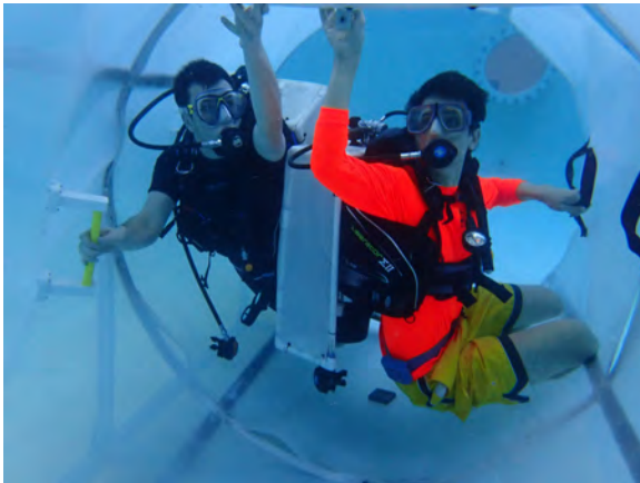
Figure 6. Dual-subject testing – note rigid handrails on left side, flexible handhold on right
