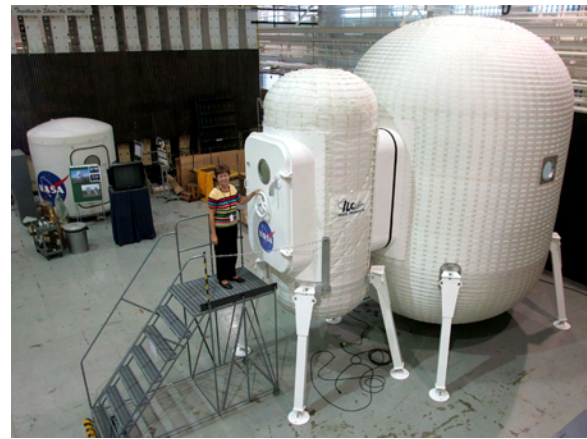
Figure 2. ILC-Dover inflatable airlock as part of inflatable habitat prototype
