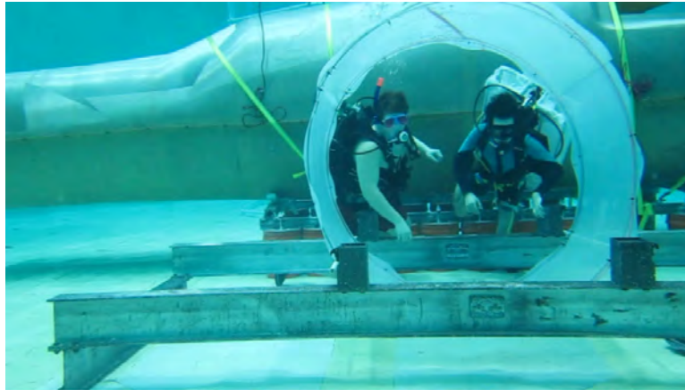
Figure 3. Neutral buoyancy investigation of required airlock diameter using resizable test fixture
