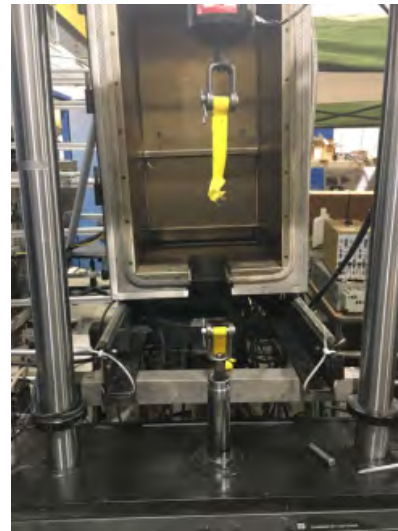
Figure 14. Pressure bladder sample post-failure in tensile testing machine
