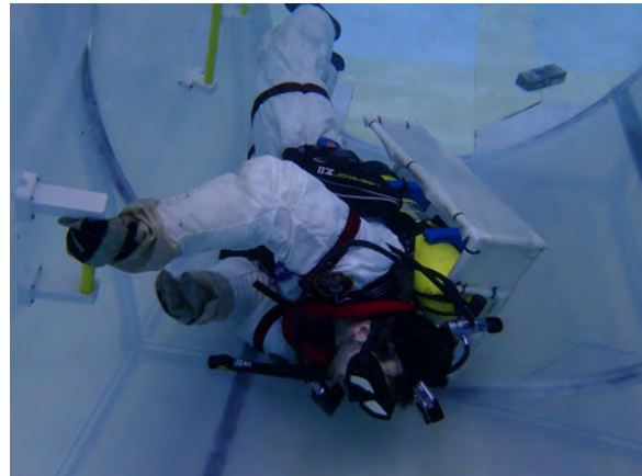
Figure 7. Airlock and hatch testing with suited subject
