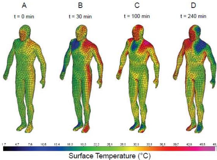
**Figure 10. Heat output and suit surface temperature varies throughout a simulated Martian EVA. [Image from Ref. 4]**
