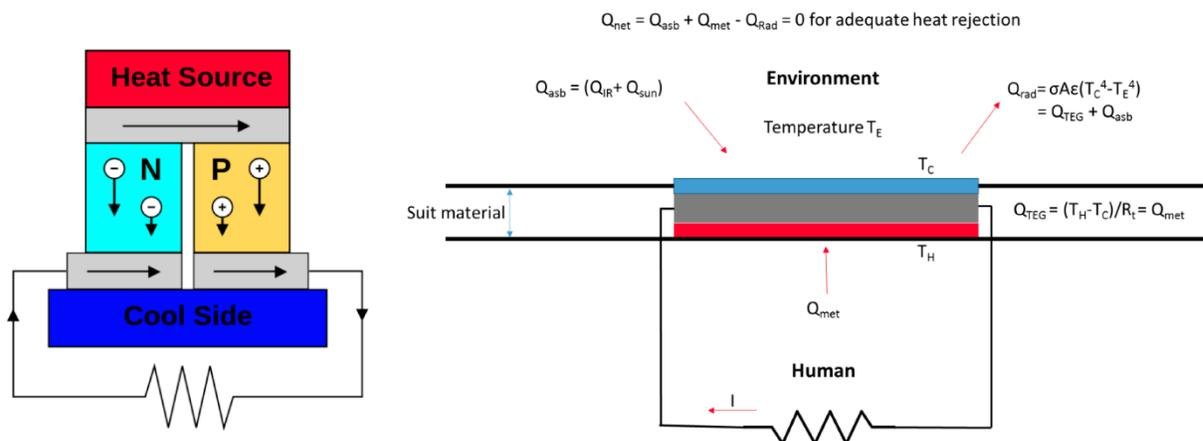
**Figure 7. Thermoelectric generator diagram and hypothetical spacesuit implementation.** In a TEG, electrons in the N-type substrate and holes in the P-type substrate migrate away from a heat source, causing a net current flow. In a thermoelectric cooler, the current is run in the opposite direction. In an EVA suit,  $Q_{net}$  (composed of metabolic heat, radiative heat, and environmental heat) should be zero for maintain a temperature setpoint within the suit [Images from Ref. 23]
