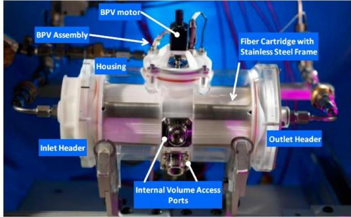
**Figure 3. Gen2 SWME.** Lab testing of the Space Water Membrane Evaporator for the xEMU. The unit is less than 50 cm long and would fit inside the PLSS backpack [Image from Ref. 17]
