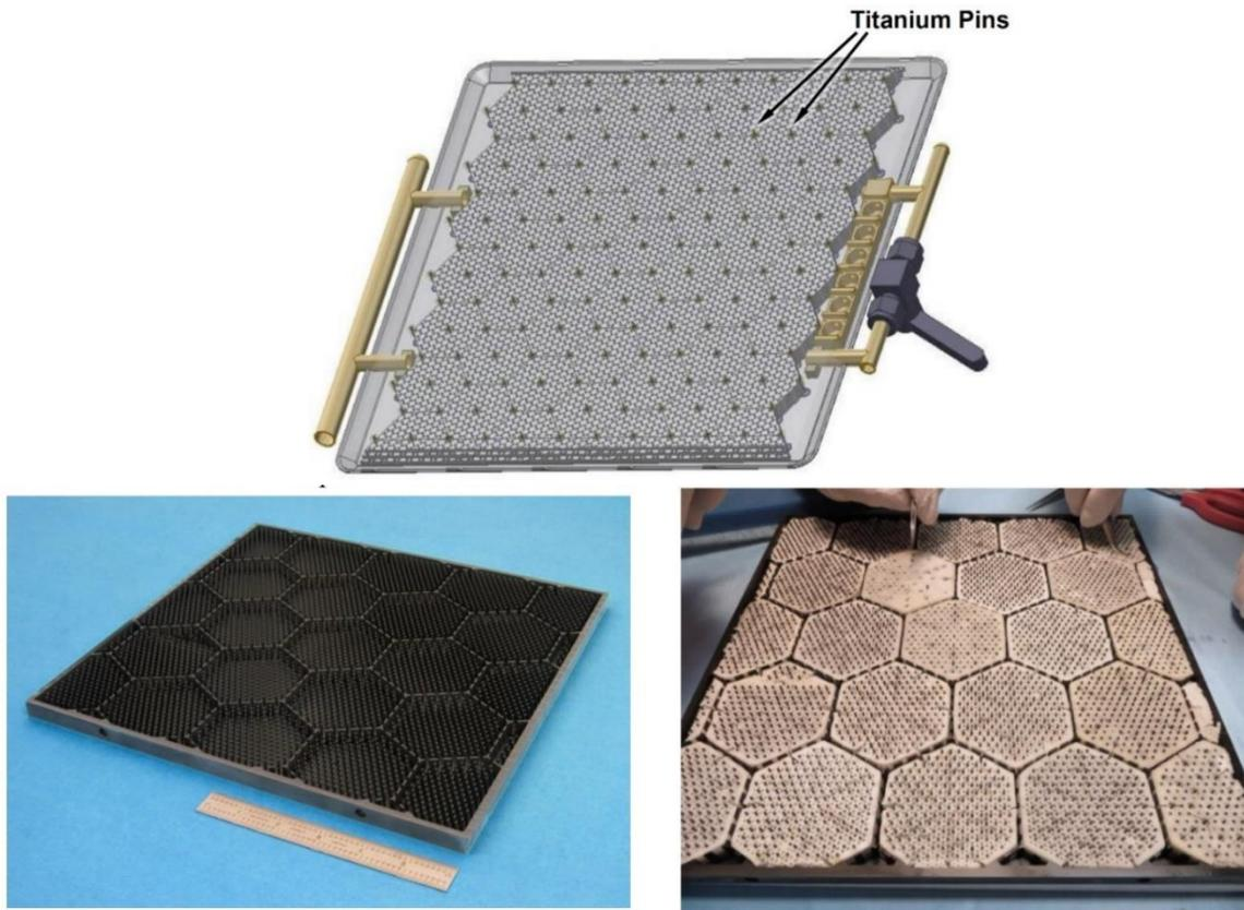
**Figure 6. Cutaway view of LCAR titanium and graphite honeycomb module, designed for integration into PLSS shell. The flight prototype is 1 ft<sup>2</sup> by 0.5 in thick. The front radiating surface (coated in high emissivity aeroglaze) is not shown. This prototype panel exhibited a 19% efficiency improvement over previous iterations during TVAC testing [Images from Refs. 18-19]**
