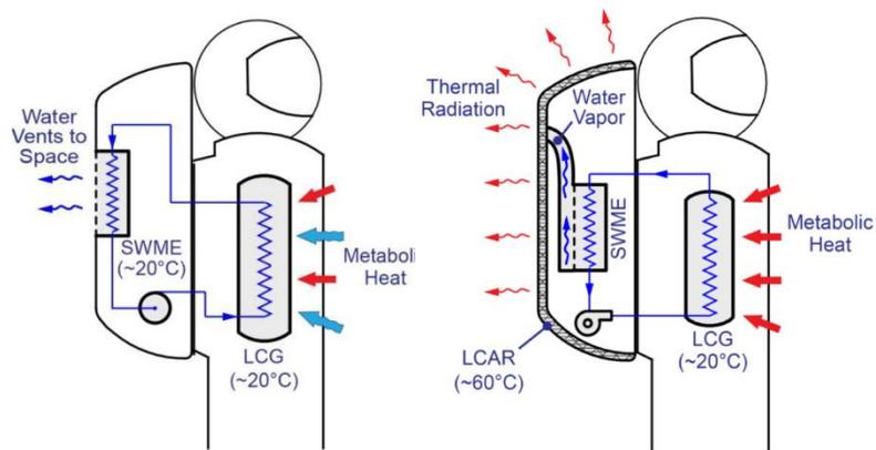
**Figure 4. Comparison of heat rejection using SWME and SEAR.** The SEAR system rejects heat by absorbing water vapor and radiating the latent heat, as compared with the SWME independent system that directly vents the water vapor [Image from Ref. 17]
