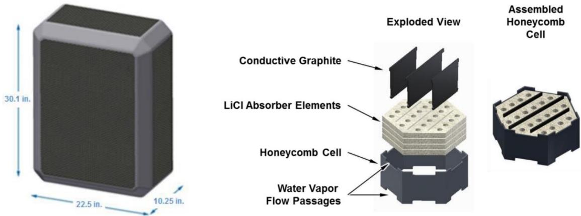
**Figure 5. Proposed honeycomb LCAR design for the PLSS backpack. [Image from Ref. 16]**
