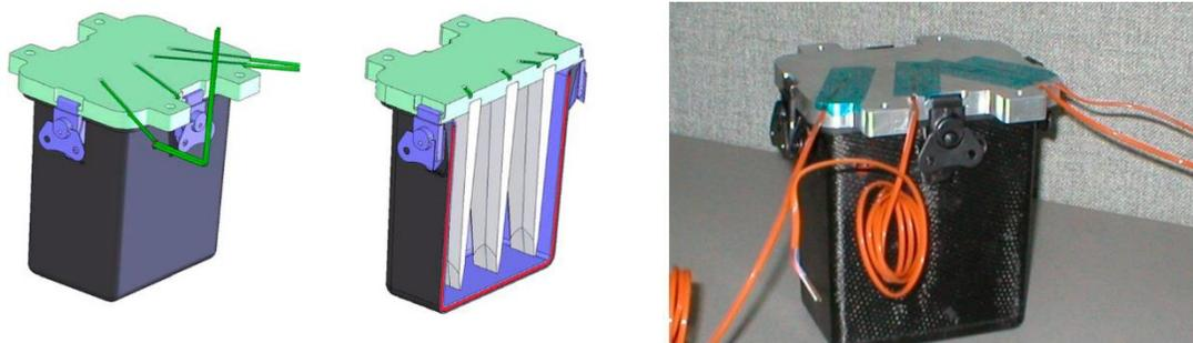
**Figure 8. Cryogenic water ice phase change material heat sink demonstrator.** *This proof of concept cooling pack is about 16.5 cm x 16.5 cm x 7.3 cm and contains about 1.85 kg of ice. The device includes a carbon composite shell, a foam liner to accommodate for thermal expansion and contraction, and metal fins for enhancing heat transfer [Images from Ref. 24]*
