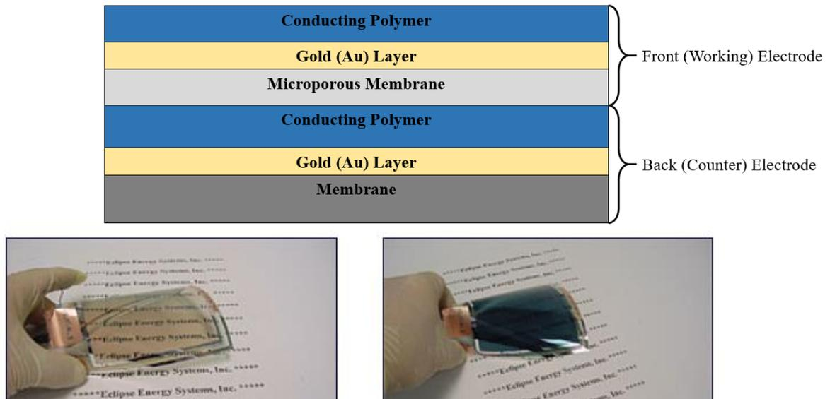
**Figure 9. Flexible thin film electrochromic demonstration by Eclipse Energy Systems. A small applied voltage can darken the color of the material and raise its thermal emissivity [Images from Refs. 28 and 30]**
