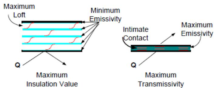
**Figure 11. Concept of internal suit lofting for conductive heat transport control.** Active shape change materials would alter suit insulation by extending or compressing the suit layers depending on heat rejection needs [Image from Ref. 25]
