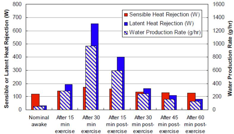
**Figure 2. Human cooling mechanisms.** *The human body rejects both sensible and latent heat. Latent heat rejection increases with activity level as perspiration and exhalation increase [Image from Ref. 11]*
