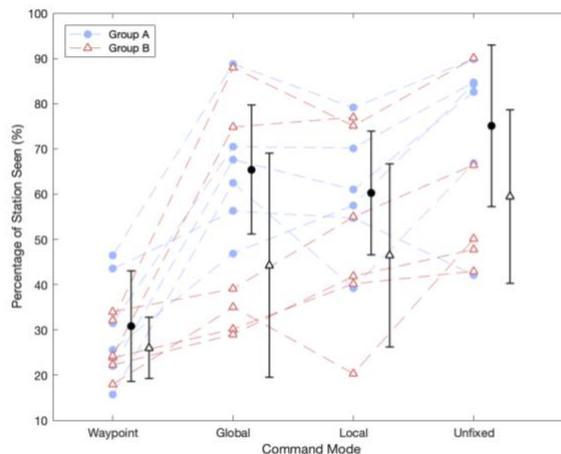
**Figure 4. Subject average percentage of station seen across command modes. Blue and red markers indicate means in Group A and B respectively. Black markers and error bars show the standard deviation from overall mean.**
