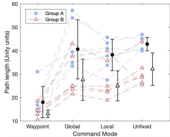
**Figure 6. Average path length across each trial. Blue markers and red markers indicate subject values in each trial within Group A and B respectively. Black markers and error bars indicate the standard deviation from the overall mean.**
