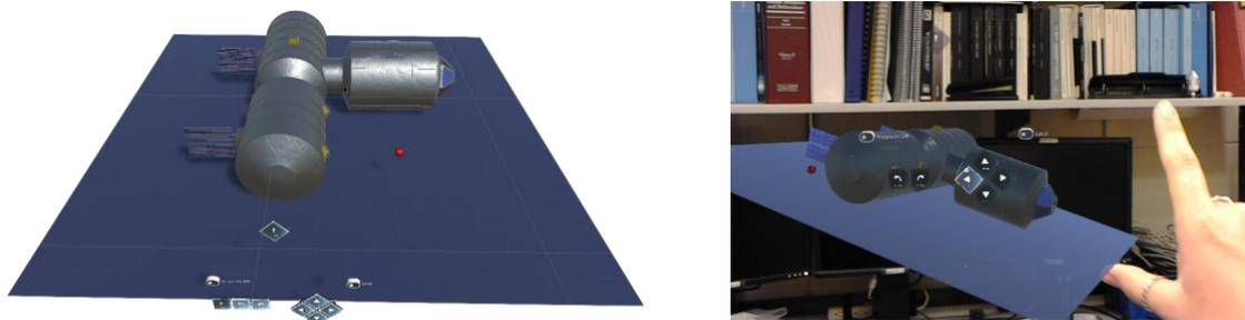
**Figure 1. (Left) Complete model of the simulation environment, showing the space station, reference plane and control pad. The inspector is shown in red. (Right) The simulation implemented on HoloLens, utilizing in-built HoloLens gestural control. Here the subject is pressing the left arrow key on the control interface to move the inspector in the  $-Y$  direction in the local frame.**
