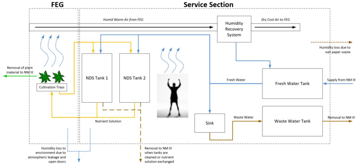
**Figure 1. Water cycle, inputs and outputs of the EDEN ISS MTF.**
