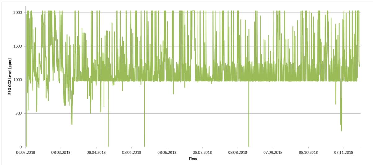
**Figure 2. FEG CO<sub>2</sub> level during the experiment phase in 2018. Note: CO<sub>2</sub> sensor range was 0-2,000 ppm. Values above 2,000 ppm were not measured.**
