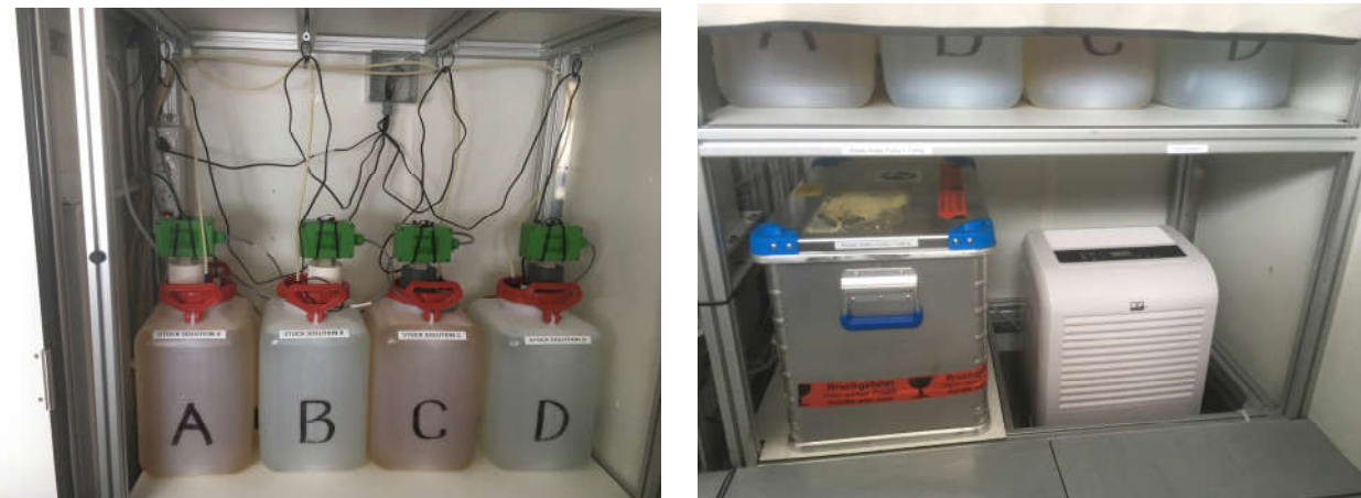
Figure 4: (Left) New stock solution bottles with level sensors. (Right) Stand-alone dehumidifier for the MTF Service Section
