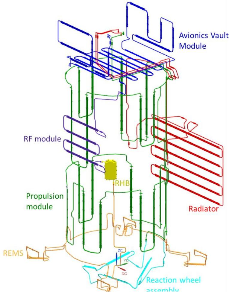
Figure 1: Europa Clipper spacecraft HRS tube layout.
