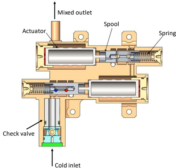
**Figure 3: Europa Clipper flight thermal control valve configuration showing two mixing valves in series. Note: the two hot inlets are not shown in this cross-sectional view.**
