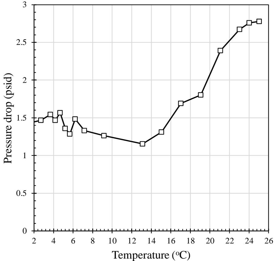
**Figure 7: Pressure drop of thermal control valve as a function of mixed fluid temperature.**
