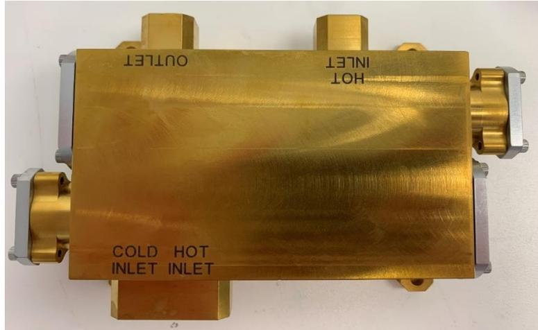
**Figure 4: Europa Clipper engineering model thermal control valve.**
