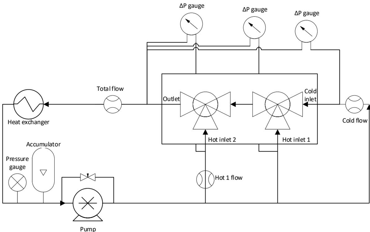
**Figure 5: Thermal control valve test loop diagram.**
