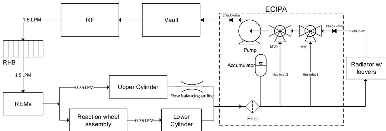
**Figure 2: Europa Clipper HRS loop diagram showing major system components and modules.**
