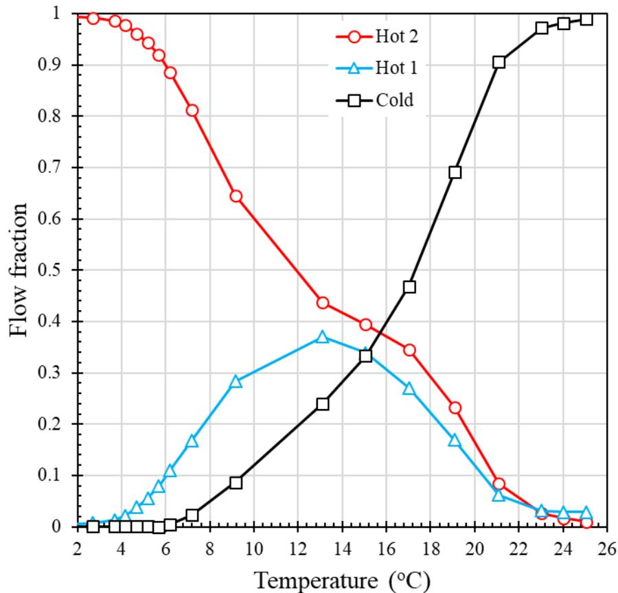
**Figure 6: Flow fraction of hot 1, hot 2, and cold inlets of the thermal control valve as a function of mixed fluid temperature.**
