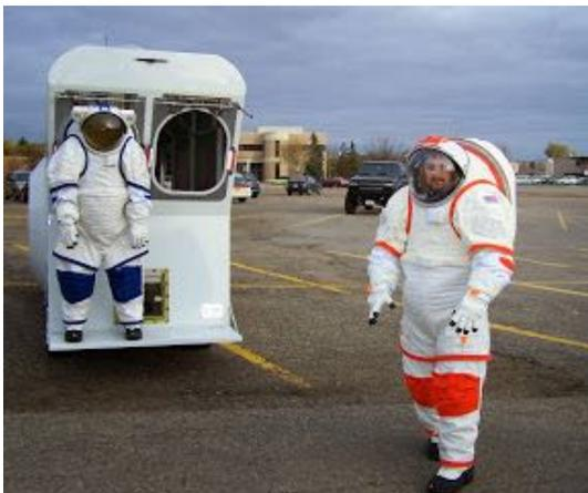
**FIGURE 4. NDX spacesuits with the UND lunar/Mars rover simulator with dual Suitports installed in the aft bulkhead. Photo credit: Pablo de Leon.**
