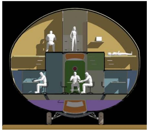
**FIGURE 6. Cross-Section through the inflatable SEIM lunar-planetary habitat module. The private sleep compartments appear in the upper left and upper right. Courtesy of Constance Adams and Georgi Petrov.**
