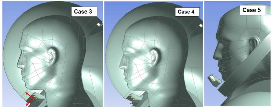
Figure 10: Position of the purge valve in cases 3-5
