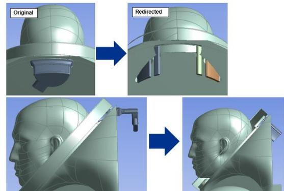
**Figure 8: Redirected inlet geometry in case 2**
