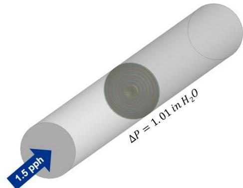
**Figure 3: Gurley model altered to determine the necessary area of the hatch port**
