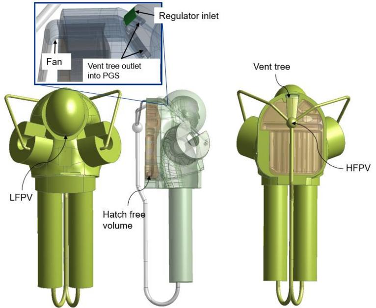
**Figure 1: Nitrogen purge design modeler geometry**
