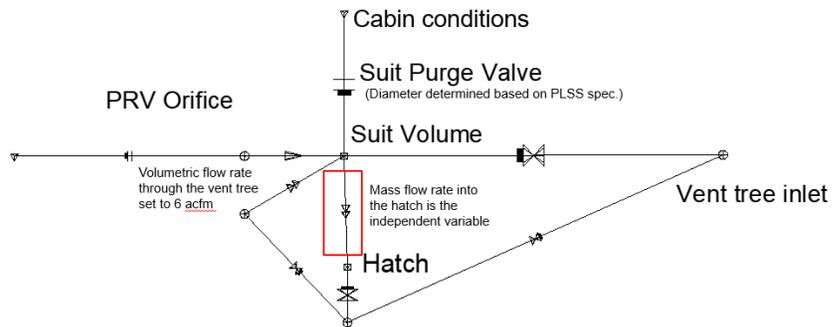
**Figure 2: FloCAD model used to size the vent tree hatch port**
