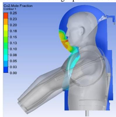
**Figure 12: Contour of concentration of CO<sub>2</sub> at the bisectional suit plane**
