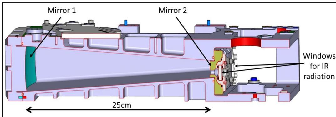
**Figure 2: Cut-view of gas cell with internal mirrors.**
