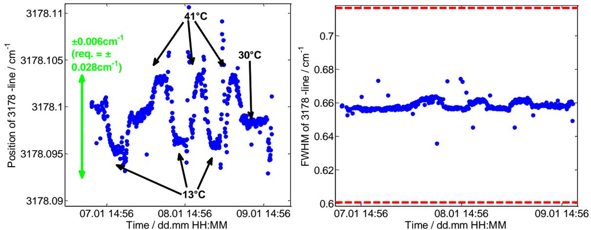
**Figure 8: Line shape parameters at temperature testing. Left: Line Position. Right: Full width at half maximum. The red lines show the required stability, where for the line shape it is at  $\pm 0,028\text{cm}^{-1}$  and therefore outside the plot ranges.**
