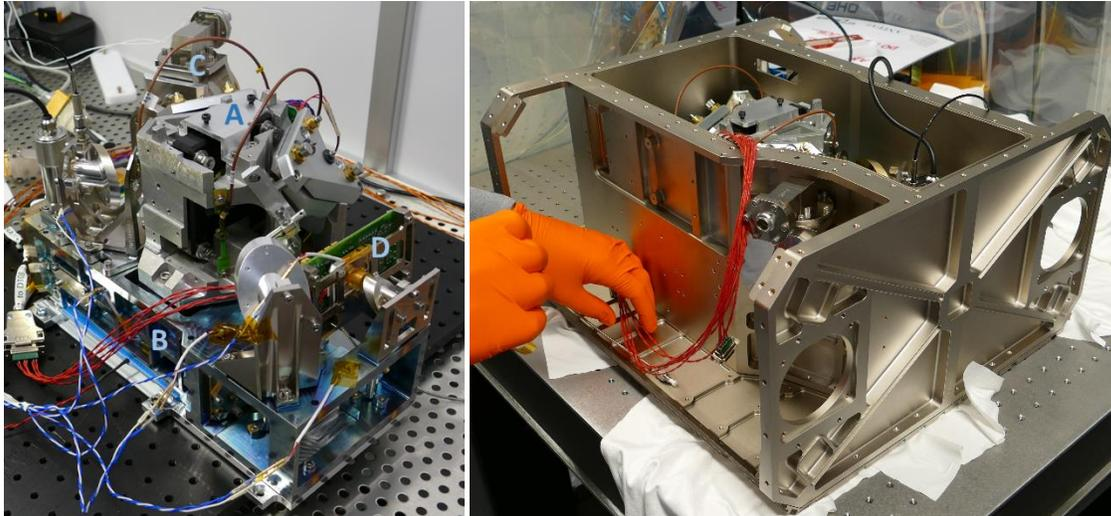
**Figure 4: Left: Aligned FM optomechanical sub-assembly (A: Interferometer, B: Gas Cell, C: IR Source, D: IR Detector). Right: optical compartment walls mounted.**
