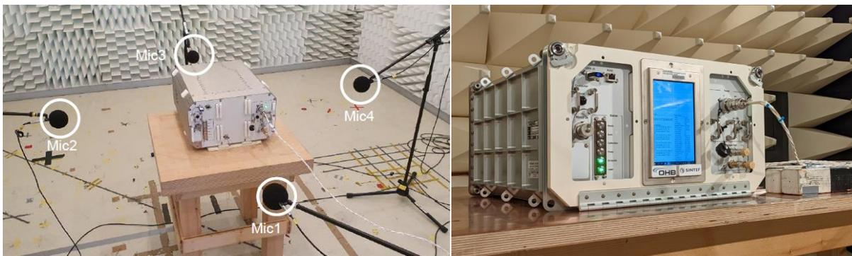
**Figure 10: Left: Setup for audible Noise Testing; Right: ANITA2 at EMC test**
