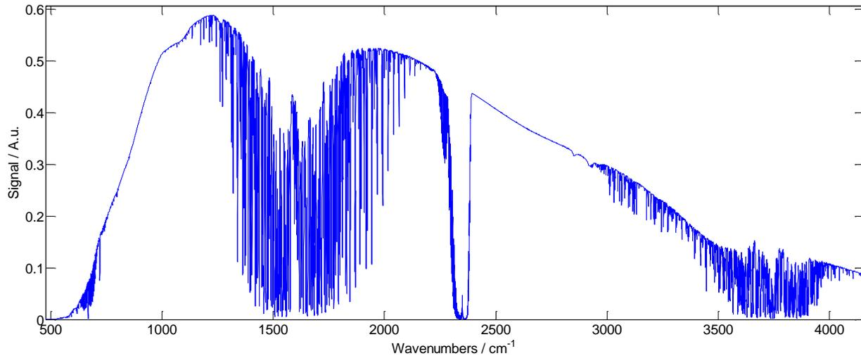
**Figure 6: ANITA2 spectrum. The applicable spectral range spans from about 650 to 4400 cm<sup>-1</sup>, which is 155 to 2.3µm.**
