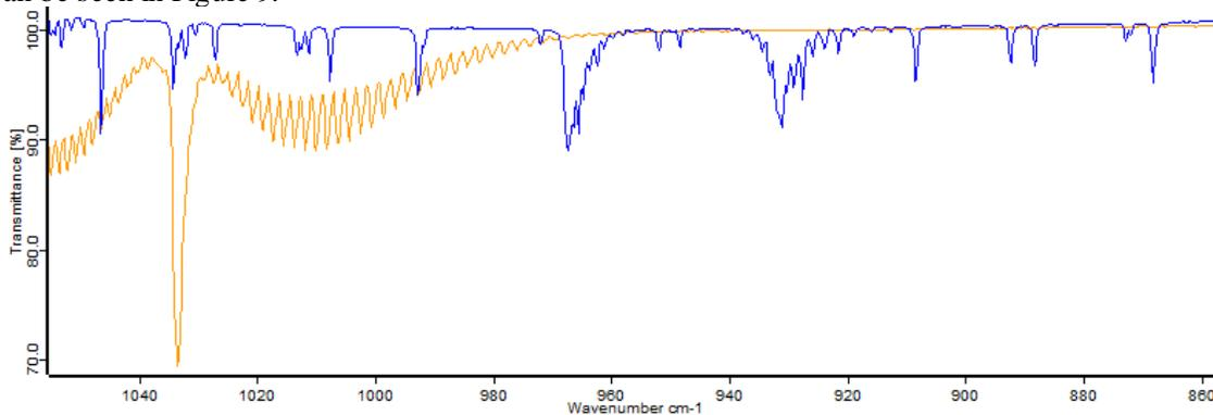
**Figure 9: ANITA2 FM spectra from 20ppm methanol (orange) and 6ppm ammonia (blue) in  $\text{N}_2$ .**
