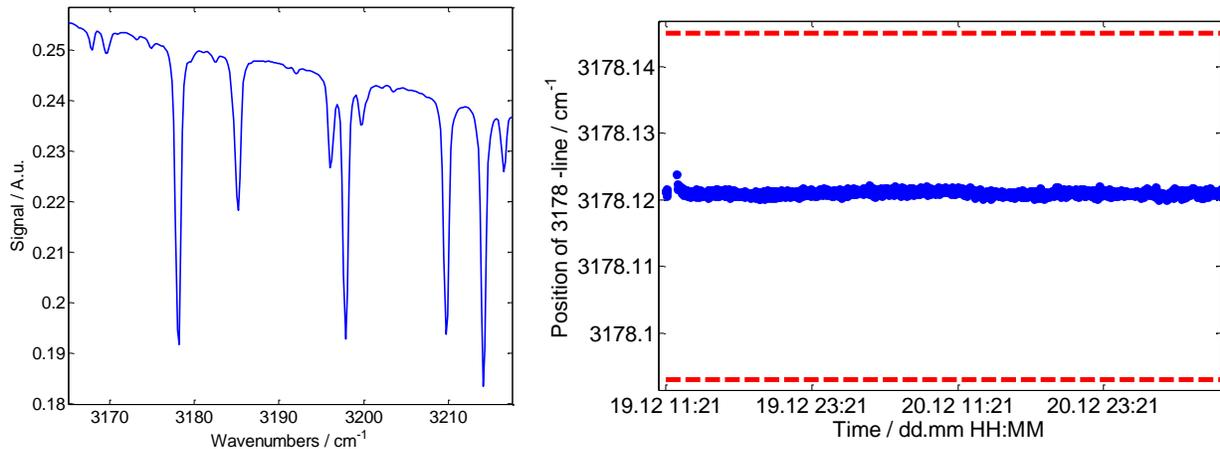
**Figure 7: Left: Zoom into Figure 6 showing water vapour lines in more detail. Right: Position stability of one line over time. The red lines show the requirement.**
