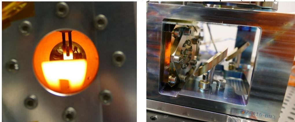
**Figure 3: Left: IR-source: Heated u-shaped element and magnified mirror image can be seen. Right: Entrance and exit optics of gas cell including entrance window mounting.**
