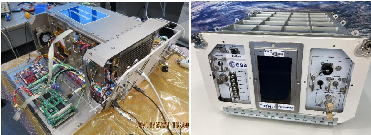
**Figure 5 Left: ANITA2 harness integration. Right: Finally assembled ANITA2 inside a MDL.**
