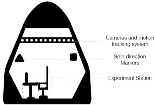
**Figure 3. Sketch of one of the possible interior configurations of the crew dragons.**
